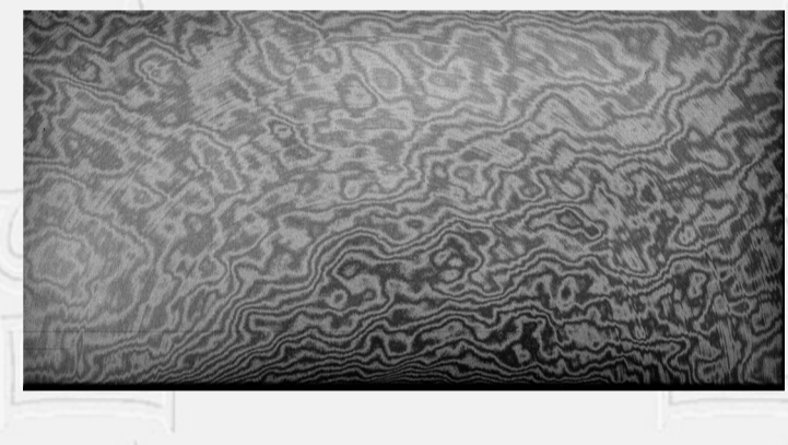
Figure 8 : Flat field (λ = 900nm, bandwidth = 5nm, 1500ADU)
