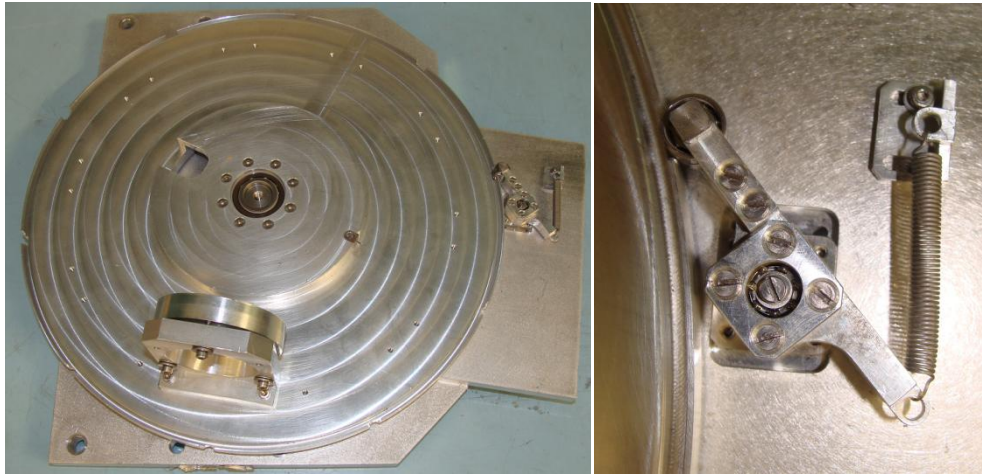
Figure 2: Spring locking system
