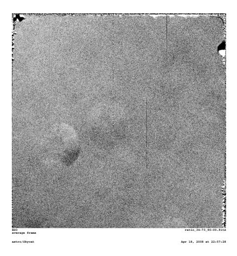
Figure 21: Ratio of dome flat fields taken at different rotator angle. The px-to-px differences are less than 1% .
