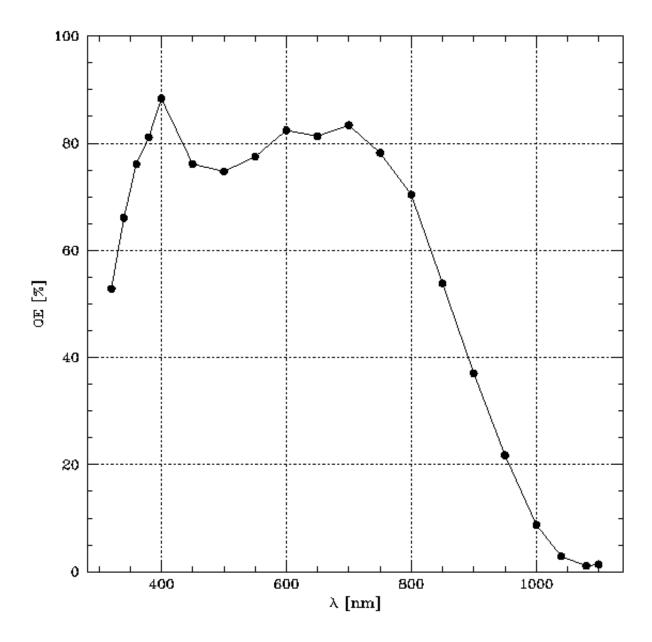
Figure 12: Quantum Efficiency of CCD#40.
