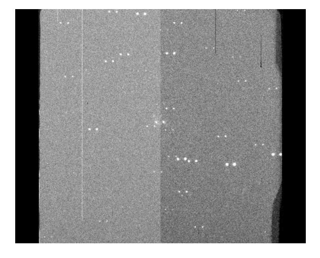
Figure 8: An image taken with the focus wedge. Each object is split into two. In this case the telescope is almost focused, since the split images are at nearly the same level with each other. Note that the fast readout using two amplifier gives the split appearance of the background.
