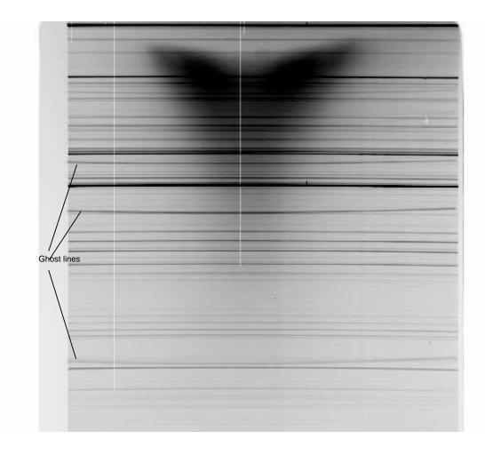
Figure 14: Artefacts in an Arc image. This is illustrated by an image of the He Ar arc lines for Grism 9. As well as the arc lines, there is reflected light from the Argon Lamp at the top of the frame. Very faint ghost lines resulted from reflection can also be seen in the image as lines which curve upwards. Both types of features do not affect the wavelength calibration as long as care is taken when identifying the lines. It must be emphasized that the ghost lines are faint.
