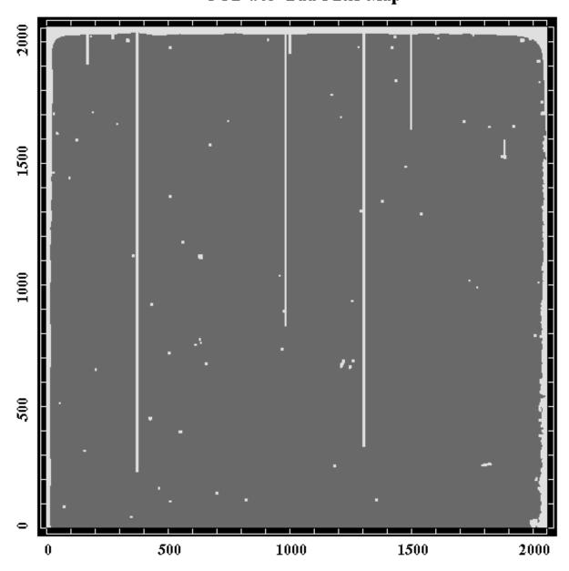
Figure 13: Bad pixel map of CCD#40. The latest bad pixel map can be found on the web.
