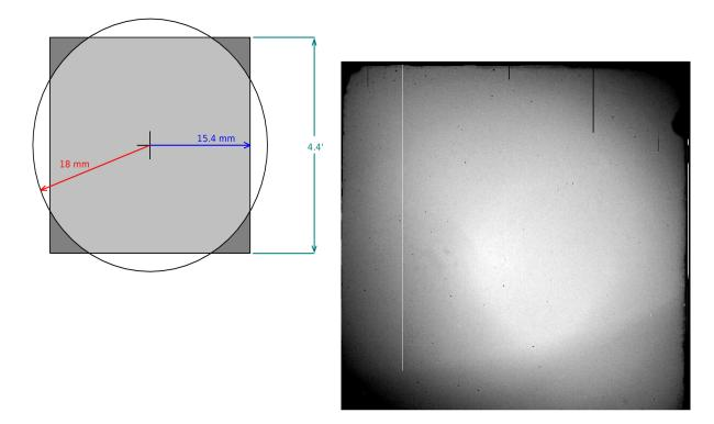
Figure 20: Left: The dark shaded area shows the regions of the detector that will be affected by some degree of vignetting, after changing to the slower f/11 ratio of the NTT. It corresponds to  $\approx 8\%$  of the active field of view. Right: a blue dome flat field after the installation of EFOSC2 at the NTT.
