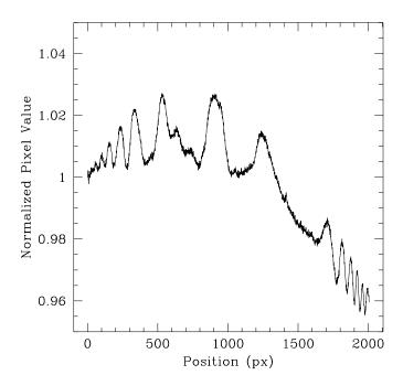
Figure 22: Upper panel: Fringe pattern on a 10 minutes exposure in the I band (CCD#40). Lower Panel: A mesh of the central 100 columns from an I superflat obtained combining 14 exposures of 480s each (courtesy of A. Iovino).
