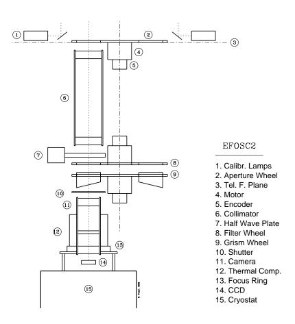
Figure 1: Schematic optical and mechanical layout of EFOSC2.
