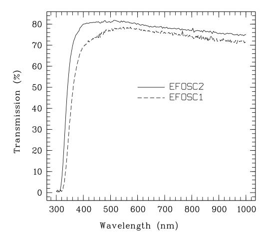
Figure 2: Overall transmission of the EFOSC2 optics compared to EFOSC1.
