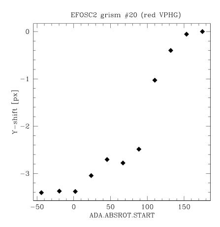
Figure 25: The shift in dispersion direction of spectra taken at different rotator angles.
