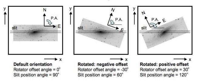
Figure 16: EFOSC2 slit orientation
