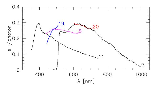
Figure 7: System efficiency given by VPHGs #19 (blue curve) and #20 (red curve) compared to that of other EFOSC2 grisms.
