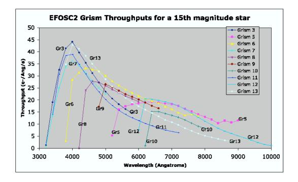
Figure 33: EFOSC2 Grism Throughputs (in electrons per Angstrom per second) for a 15th magnitude star. These represent the averaged values of different observations of many spectrophotometric standard stars, normalized to 15th magnitude at all wavelengths.
