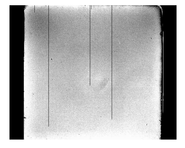
Figure 17: Normalized R dome flat field (September 2003). The image cuts are 0.96,1.04. The scratches on the left side of the detector are due to the support of the Movable slit. The spot in the center is due to the Sky Concentration.
