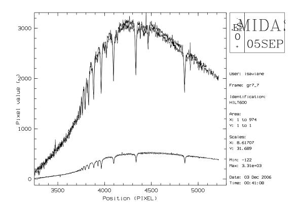
Figure 6: ADU  $\sec^{-1}$  vs. wavelength for the two spectrophotometric standards Hiltner 600 (top spectrum) and LTT 2415. For each standard the two spectra have been taken with grisms nr.7 and 14.
