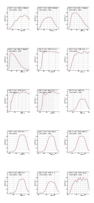
Figure 3: Laboratory transmission curves of the EFOSC2 standard set of filters. Note although they are labelled SUSI they are instrument independent.
