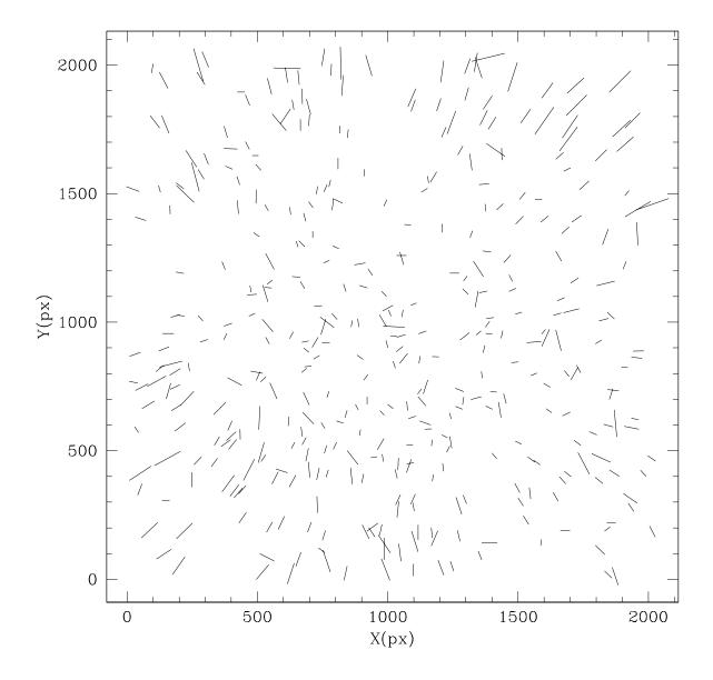
Figure 18: The PSF shape variation across the CCD. It is measured by determining the PSF ellipticities in an image of the loose globular cluster Pyxis stellar fields taken under good seeing (< 0.75 arcsec) conditions. The vectors indicate the orientation and magnitude of the PSF ellipse at that CCD location.
