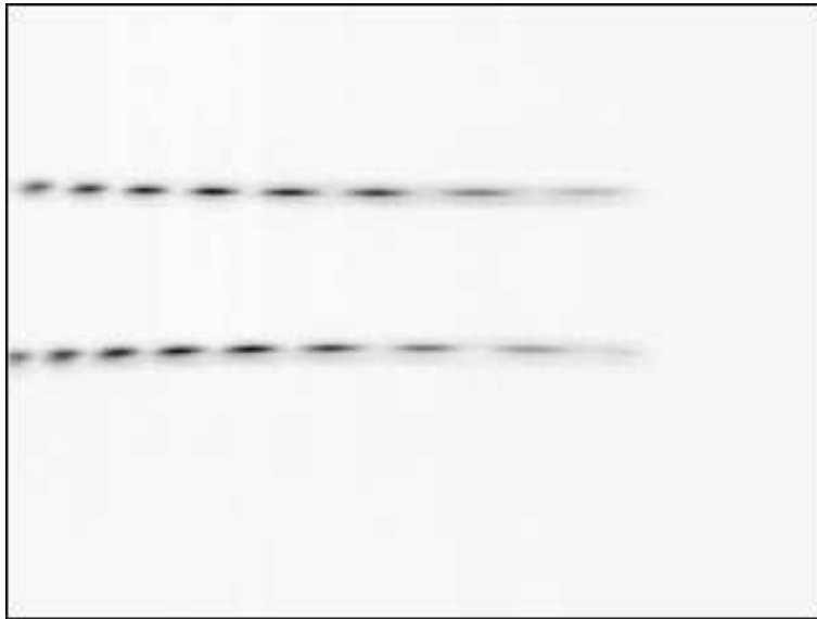
Figure 6: Image of dispersed fringes obtained in laboratory by MIDI with its grism.
