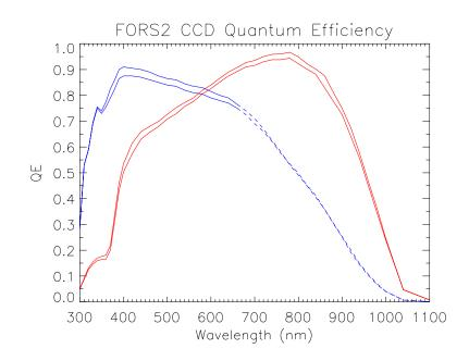
Figure 2.6: Quantum efficiency of the MIT (red) and E2V (blue) CCDs. The individual curves show the slight difference in QE of the 2 detectors in each mosaic. The dashed line shows where the fringing will limit the S/N achievable with the E2V detector.
