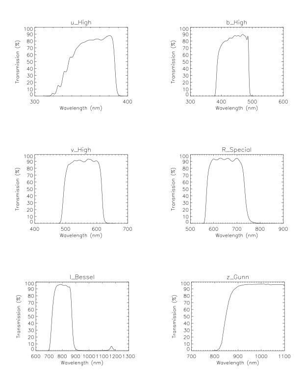
Figure B.1: Filter transmission curves for the standard instrument broadband filters.
