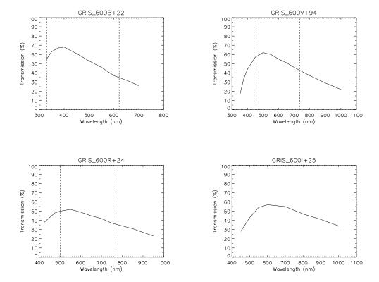
Figure C.2: Efficiency curves of the medium resolution grisms. The vertical lines mark the approximate limits of the spectral range with the slit in the center of the field.
