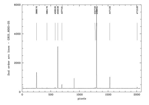
Figure D.11: 2nd order calibration spectrum taken with the SR collimator and grism GRIS\_600I+25
