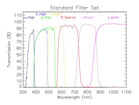
Figure 2.3: The FORS2 filters which can either be used in the ubvRIz sequence or the ugrIz sequence to cover the full wavelength range with broad band filters.
