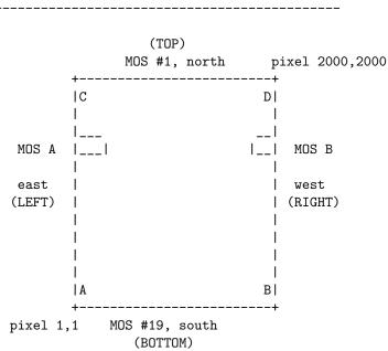
MOS Orientation and CCD Read-out Ports Rotator angle = 0 (position angle on sky = 0)
