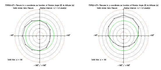
Figure 2.4: Results of flexure measurements as a function of the rotator position for the SR collimator at zenith distance of  $40^{\circ}$ . The panels show the flexure in *un-binned* pixels across (X) and along (Y) the slit. The solid green circle represents zero-flexure.
