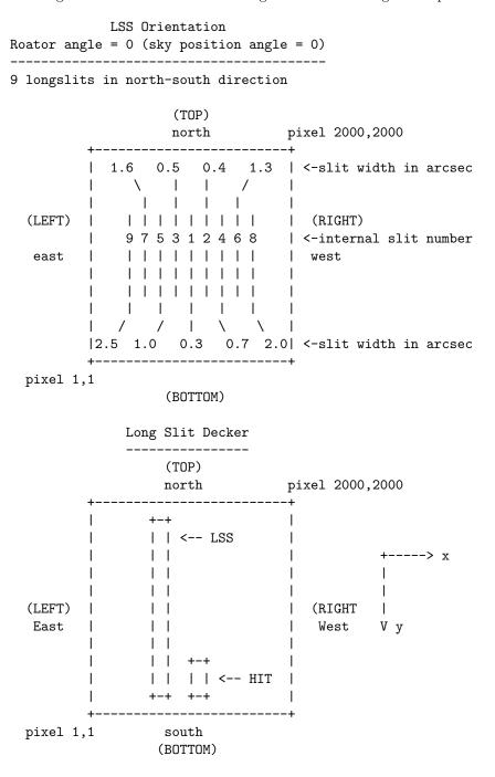
The x-distance between HIT decker and LSS decker is half the distance between two LSS slits. If HIT decker enables 0.3'' slit, the LSS decker will enable the large pinhole close to the center of the field of view.
