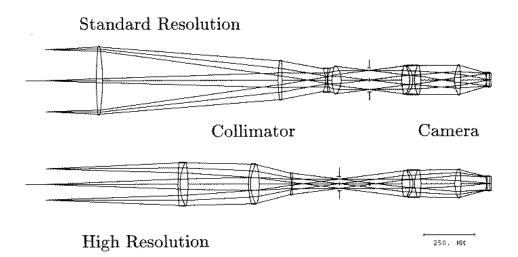
Figure 2.2: Light paths for the standard and high resolution collimators.
