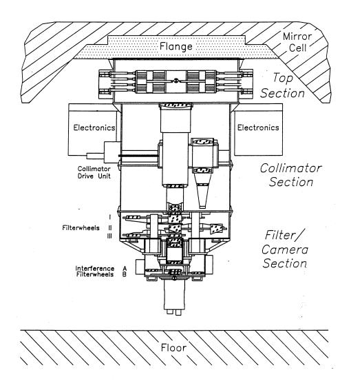
Figure 2.1: Schematic view of the FORS instruments
