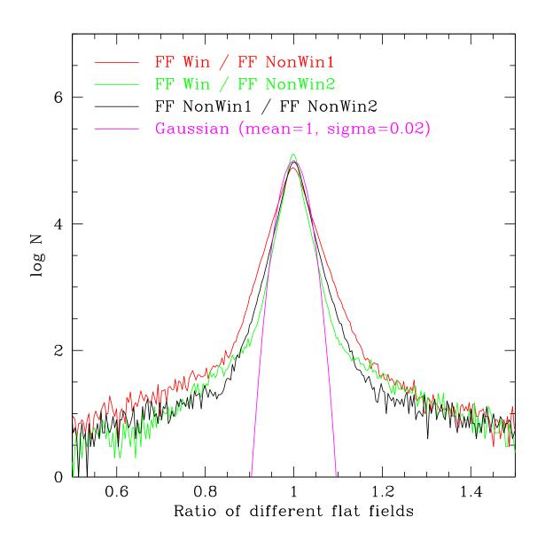
Figure 14: Histograms of the ratios between a windowed and two non-windowed  $K_S$  twilight flats. For comparison, the ratio of the two non-windowed flats and a Gaussian function is also shown.
