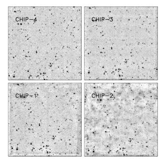
Figure 11: The field around the z=2.7 quasar B0002-422 as seen in the 4 HAWK-I quadrants. Radioactivity effects are clearly visible in Q 2 (chip #78)
