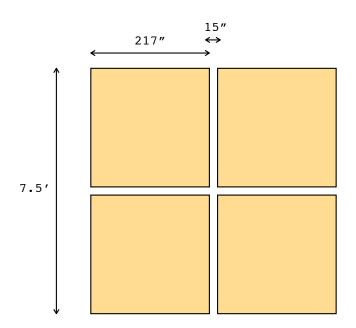
Note that it is very tempting to point *right onto* your favourite target and to loose it in the gap, since this is where the telescope points.
