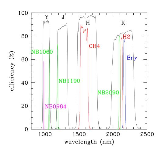
Figure 6: HAWK-I Filters. Black: broad-band filters Y, J, H, K<sub>s</sub>, Green: cosmological filters NB1060, NB1190, NB2090; Red: CH4, H2; Blue:  $Br\gamma$ ;magenta: visitor filter NB0984
