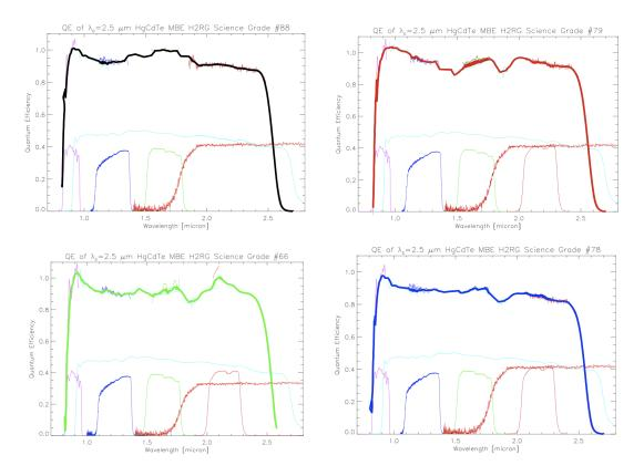
Figure 7: Quantum efficiency of the HAWK-I detectors
