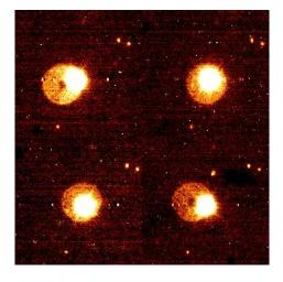
Figure 5: Smoothed enhanced images of the optical ghosts visible in the four quadrants for the NB1060 (left) & NB1190 (right) filters
