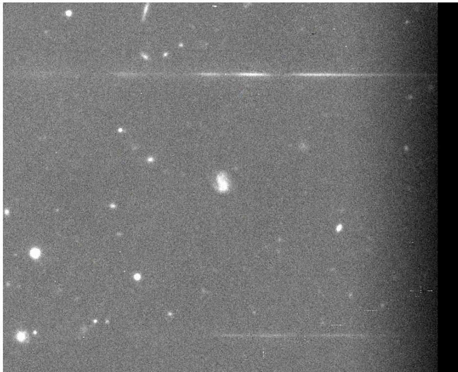
Figure 16: Example of reflection of light from a star (in this case, two stars to the West) outside the field. Such features can occur on each of the four corner CCDs.
