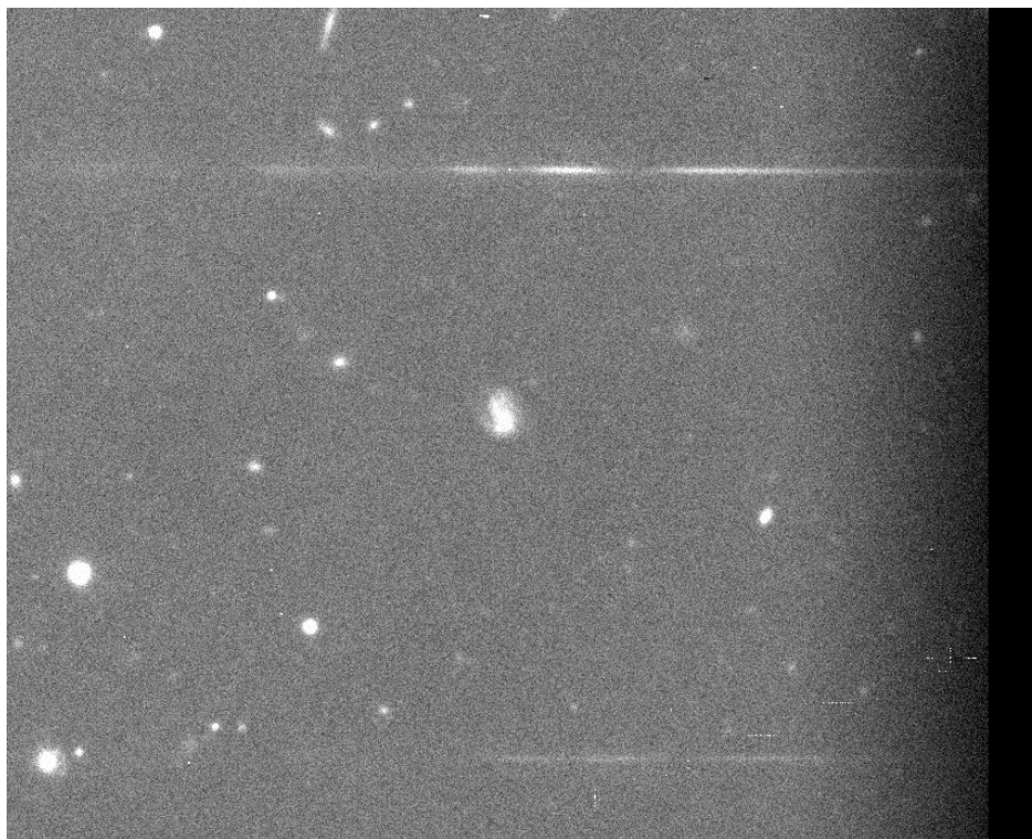
Figure 22: Example of reflection of light from a star (in this case, two stars to the West) outside the field. Such features can occur on each of the four corner CCDs.
