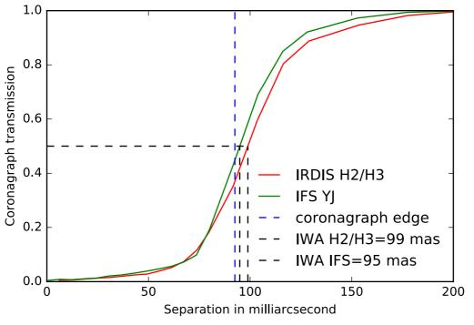
Figure 41 Transmission profile for the N\_ALC\_JYH\_S coronagraph
