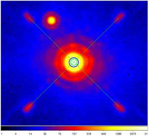
Figure 43 Non coronagraphic image of a star (happening to have a binary companion) in broadband H with Irdis, after applying a waffle pattern to the DM for calibration purposes. The green thick circle indicates the intersection of the green lines, while the blue thick circle indicates the star position (Gaussian fit). Both agree within 2.5mas.
