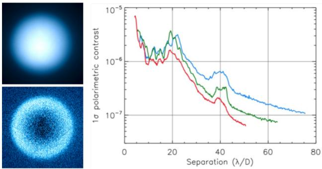
Figure 22: Top left: intensity image of Titan. Bottom Light: polarized intensity. Right: polarimetric contrast (right) on a bright target for the V (blue), N\_R (green), N\_I (red) filters.
