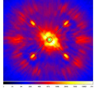
Figure 42. Irdis image in broad-band H, with the N\_ALC\_YJH coronagraph, with the waffle pattern applied to the DM, creating four satellite spots. These spots are elongated with broad-band filters and point source with narrow-band filters. The green lines start and end points were computed by fitting a 2D Gaussian on each spot, they intersect on the star center, indicated by a green thick circle.
