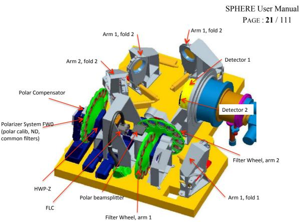
Figure 8: ZIMPOL schematic view showing the main elements of this visible polarimeter, from polarization compensator, common filter wheel, Ferroelectric Liquid Crystal (FLC) modulator to the splitter, filter wheels 1 and 2, and the two detectors.
