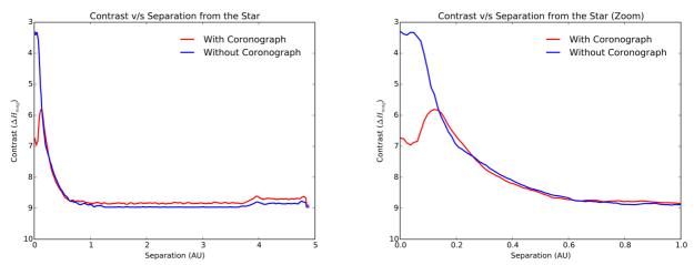
Figure 13: Contrast obtained with and without the use of the coronograph. Contrast is in H band magnitudes. Right: zoom for separations less than 1".
