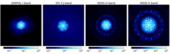
Figure 23: SAM\_7H on-sky point spread functions for 4 observing wavelengths with 3 cameras: a ZIMPOL I band exposure, a IFS wavelength slice between Y and J bands, an IRDIS H band image and an IRDIS Ks band image.
