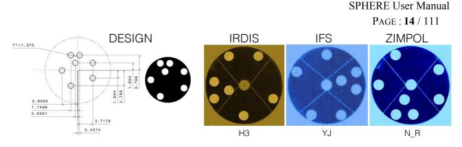
Figure 3: Layout of the SPHERE 7-hole aperture mask design projected on the 8m primary mirror. Each pair of holes (baseline) produces a set of interference fringes. The three images on the right are how the holes are located with respect to the full pupil of the telescope as seen by the 3 instruments. In the case of IRDIS, the mask has been mounted with a 90° offset and one of the holes is tangent with the telescope spider.
