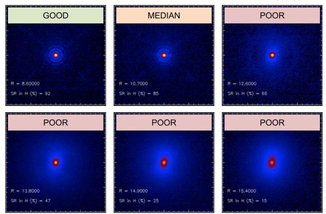
Figure 12: SPHERE PSF morphology and Strehl ratio as a function of R magnitude (see Table 10 and Table 11 for details).
