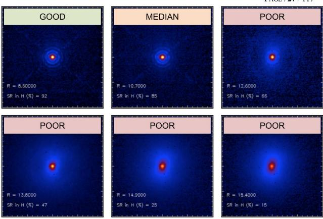
Figure 12: SPHERE PSF morphology and Strehl ratio as a function of R magnitude (see Figure 31 and Figure 32 for more details).
