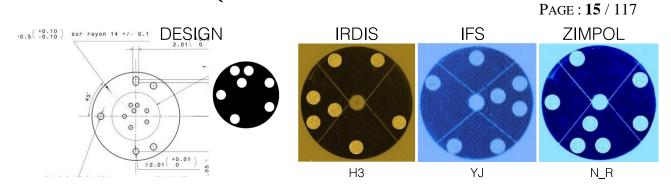
Figure 3: Layout of the SPHERE 7-hole aperture mask design projected on the 8m primary mirror. Each pair of holes (baseline) produces a set of interference fringes. The three images on the right are how the holes are located with respect to the full pupil of the telescope as seen by the 3 instruments. In the case of IRDIS, the mask has been mounted with a 90° offset and one of the holes is tangent with the telescope spider.
