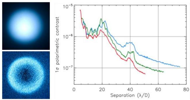
Figure 23: Top left: intensity image of Titan. Bottom Light: polarized intensity. Right: polarimetric contrast (right) on a bright target for the V (blue), N\_R (green), N\_I (red) filters.
