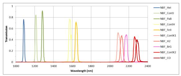
Figure 46: IRDIS NB filters.
