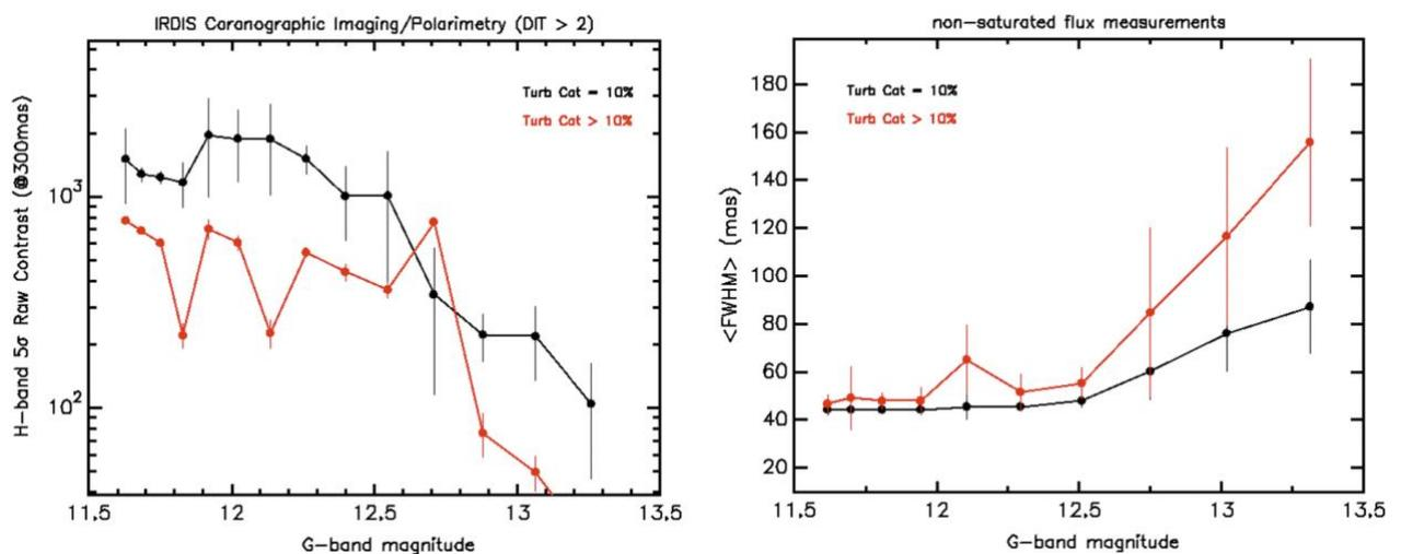
Figure 13: (Left) Single image IRDIS contrast versus Gmag. (Right) PSF core FWHM versus Gmag. Both H-band contrast and image resolution degrade quickly for targets fainter than G=12.5.
