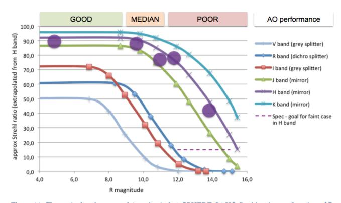
Figure 11: Theoretical and measured (purple circles) SPHERE-SAXO Strehl ratio as a function of R magnitude for good seeing conditions and different wavelength ranges from V to K (see Figure 31 and Figure 32 for more details).
