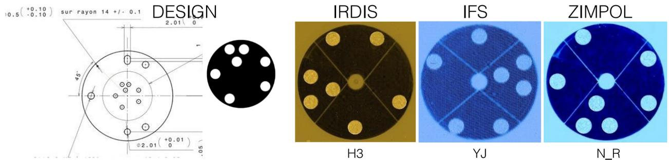
Figure 3: Layout of the SPHERE 7-hole aperture mask design projected on the 8m primary mirror. Each pair of holes (baseline) produces a set of interference fringes. The three images on the right are how the holes are located with respect to the full pupil of the telescope as seen by the 3 instruments. In the case of IRDIS, the mask has been mounted with a 90° offset and one of the holes is tangent with the telescope spider.
