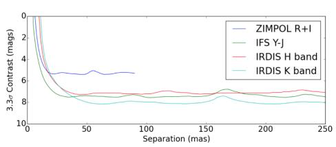
Figure 26: SAM\_7H contrast limits for the detection of companions in various bands from the test data (July 2015). Each dataset consisted of approximately 1hr in execution time, including time for observations of calibrator stars. This was obtained on the F6 star HD142527 with R=8.3, J=6.5, H=5.7, K=4.98 with a seeing ~0.6-0.8". HIP113246 and HD169319 were used as calibrator stars (Cheetham et al., in prep.).
