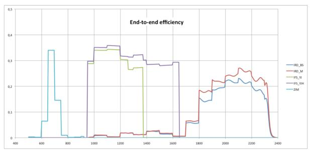
Figure 39: Transmission (as above) with different beamsplitters. In visible: separation between WFS and ZIMPOL uses a dichroic sending more light to ZIMPOL but in R band only; in NIR: the IFS/IRDIS dichroic 'K' feeds IFS with the its full Y-H range, with lower efficiency for IRDIS in K band only.
