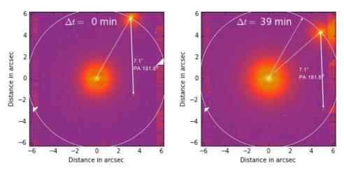
Figure 43: IRDIS ghost appears when there is a bright source on upper right corner of detector.
