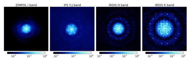
Figure 24: SAM\_7H on-sky point spread functions for 4 observing wavelengths with 3 cameras: a ZIMPOL I band exposure, a IFS wavelength slice between Y and J bands, an IRDIS H band image and an IRDIS Ks band image.
