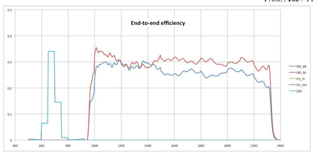
Figure 40: Transmission (as above) in IRDIS alone configuration where all the NIR light is sent to IRDIS.
