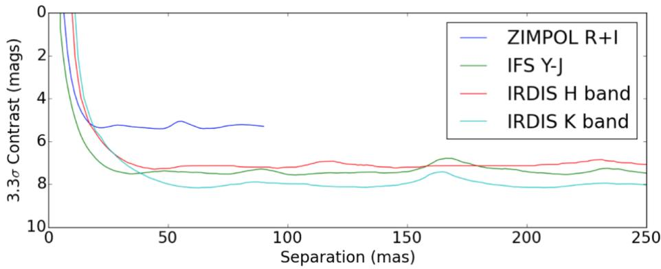
Figure 26: SAM\_7H contrast limits for the detection of companions in various bands from the test data (July 2015). Each dataset consisted of approximately 1hr in execution time, including time for observations of calibrator stars. This was obtained on the F6 star HD142527 with R=8.3, J=6.5, H=5.7, K=4.98 with a seeing  $\sim 0.6-0.8''$ . HIP113246 and HD169319 were used as calibrator stars (Cheetham et al., in prep.).
