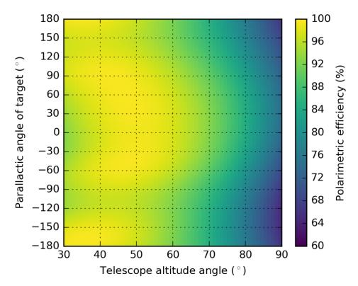
Figure 32b: Polarimetric efficiency for pupil-tracking in H-band as a function of parallactic and altitude angle (van Holstein et al. 2017, SPIE)
