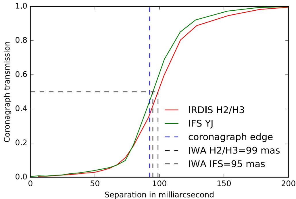
Figure 48 Transmission profile for the N\_ALC\_JYH\_S coronagraph
