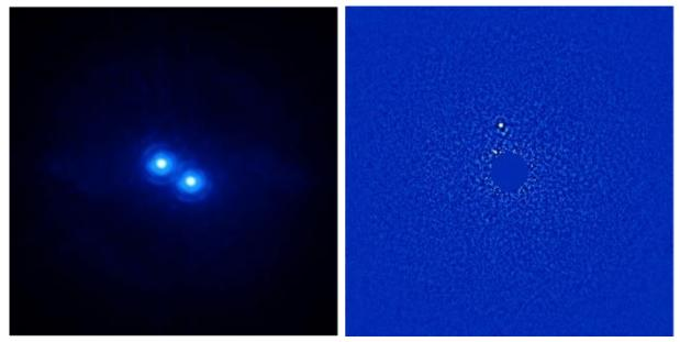
Figure 22: Left: High angular resolution imaging of a binary (150 mas separation) as seen by ZIMPOL in I band. Right: Pupil-stabilized ZIMPOL imaging providing ADI contrast close to 12 mag at 0.2" (previously unknown companion).
