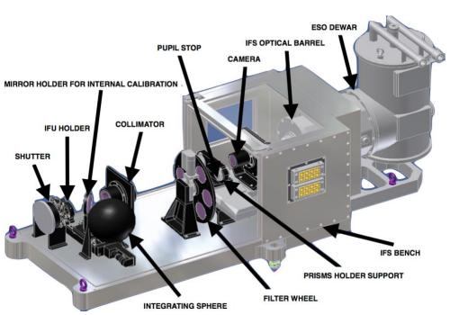
Figure 5: Inside the IFS. Note that the IFS optical bench is not cold, and that it has its own Lyot stop and internal calibration sources.
