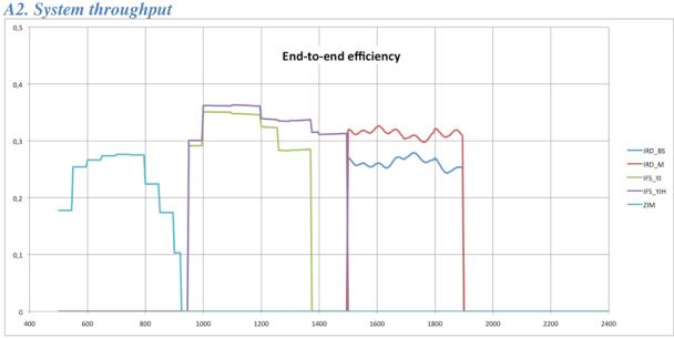
Figure 38: Transmission from SPHERE entrance to the science detectors, including the detector efficiency, assuming i) no coronagraph, ii) ZIMPOL path goes through the GREY beamsplitter (80% to ZIMPOL), and iii) the H dichroic separating the flux between IFS (up to 1450 nm) and IRDIS. Note that IRDIS cannot observe in K band in this setup.
