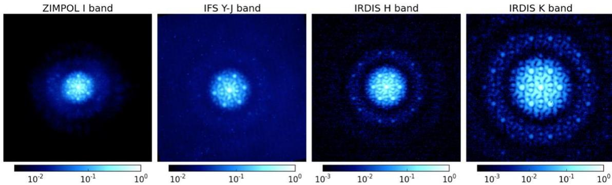
Figure 24: SAM\_7H on-sky point spread functions for 4 observing wavelengths with 3 cameras: a ZIMPOL I band exposure, a IFS wavelength slice between Y and J bands, an IRDIS H band image and an IRDIS Ks band image.
