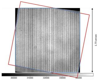
Figure 6: IFS flat-field and projection of the sky on the BIGRE detector (red) and  $\sim$ 1.73" x 1.73" FOV (blue).
