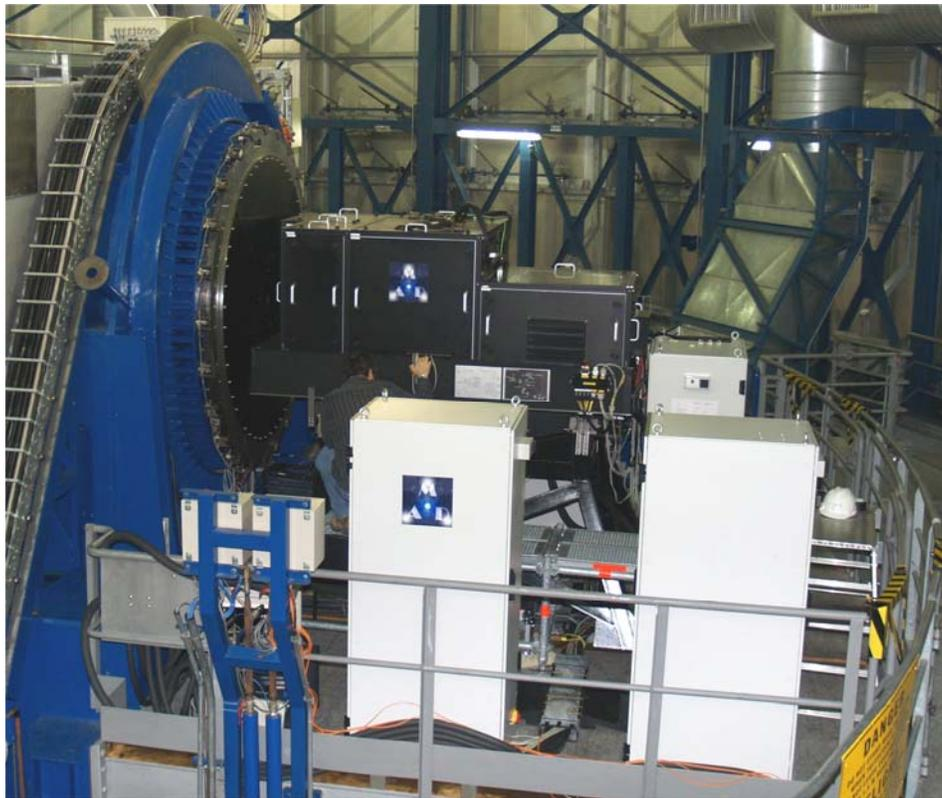
Fig. 1. The MAD bench installed at the Nasmyth focal platform of the VLT unit telescope Melipal (UT3)
