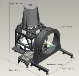
Figure 6: ASSIST Test Bench. The left-hand part is called "DSM-tower" and shows the DSM M2-Unit mounted on it. The right hand side ring structure matches the VLT Nasmyth mechanical interface and will receive the AO modules under test. A source module including a turbulence generator is shown between the DSM-tower and the Nasmyth mech. Interface.
