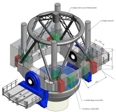
Figure 5: Mechanical layout of a VLT 8m telescope showing in green and red the cabinet space reserved for laser and its electronic implementation; grayed out volumes represent handling safety zones. The 4 large tubes on the corner represent the launch telescopes and their baffle tubes.
