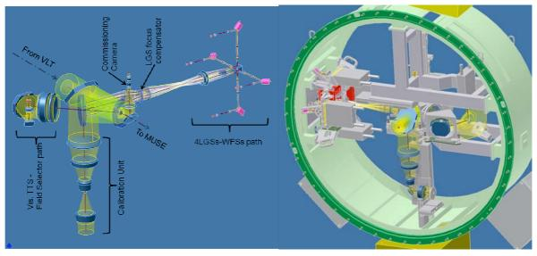
Figure 2 : The optical layout (left) and 3D mechanical model (right) of GALACSI.
