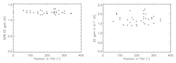
Figure 7: Gain in the size of 50% EE (left) and gain in the energy in 100 mas (right) as a function of position in the field, in K-band.
