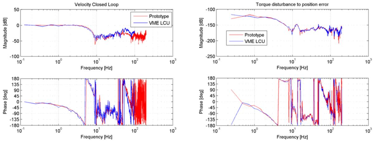
Figure 9. Closed loop velocity and position transfer function of prototype controller (left) vs. original controller (right).
