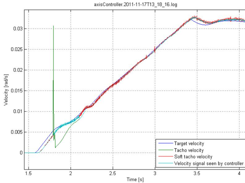
Figure 6. Behaviour of dynamical switch to work around tachometer problem.
