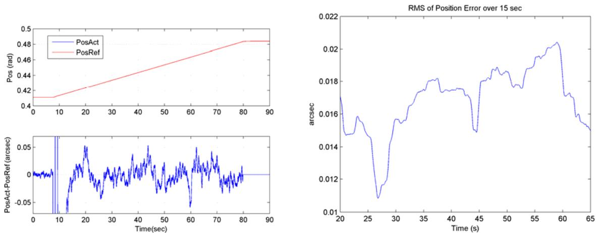
Figure 10. Time response of closed loop UT azimuth axis to ramp command.
