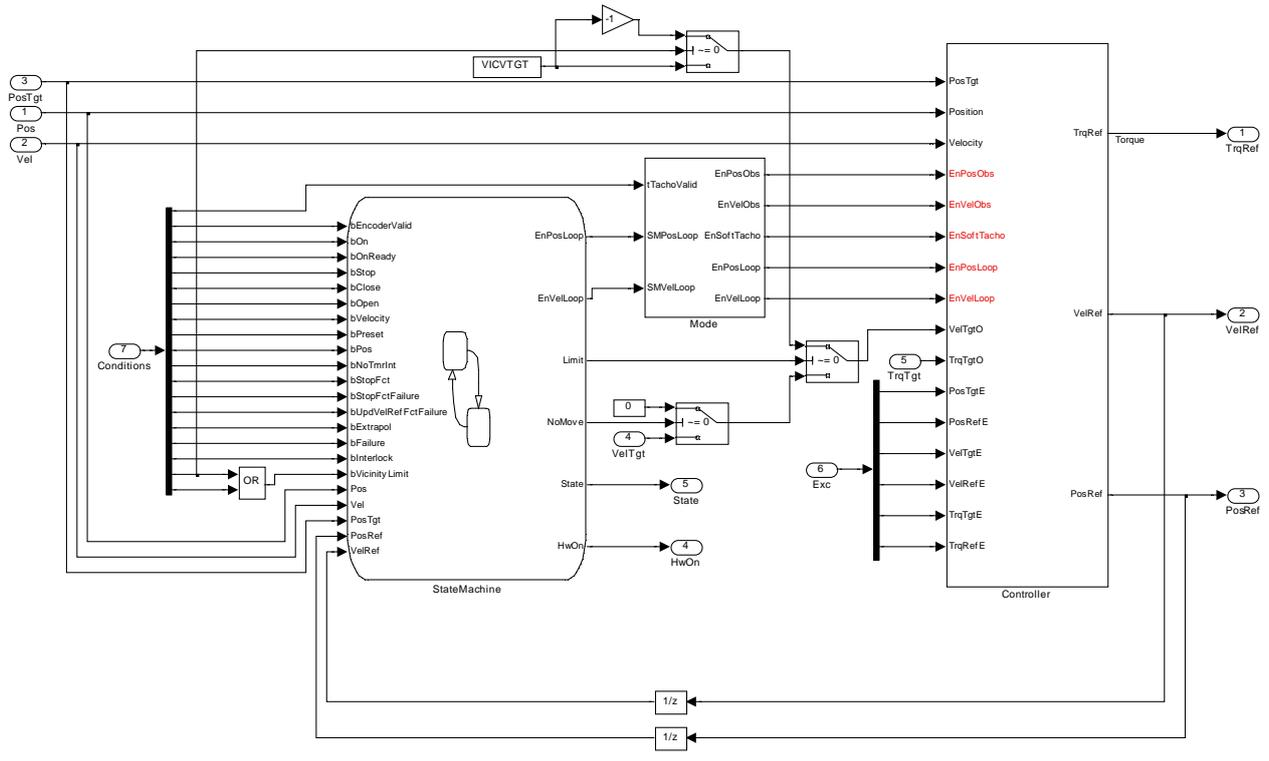
Figure 2. Simulink/Stateflow model of the controller with statemachine.
