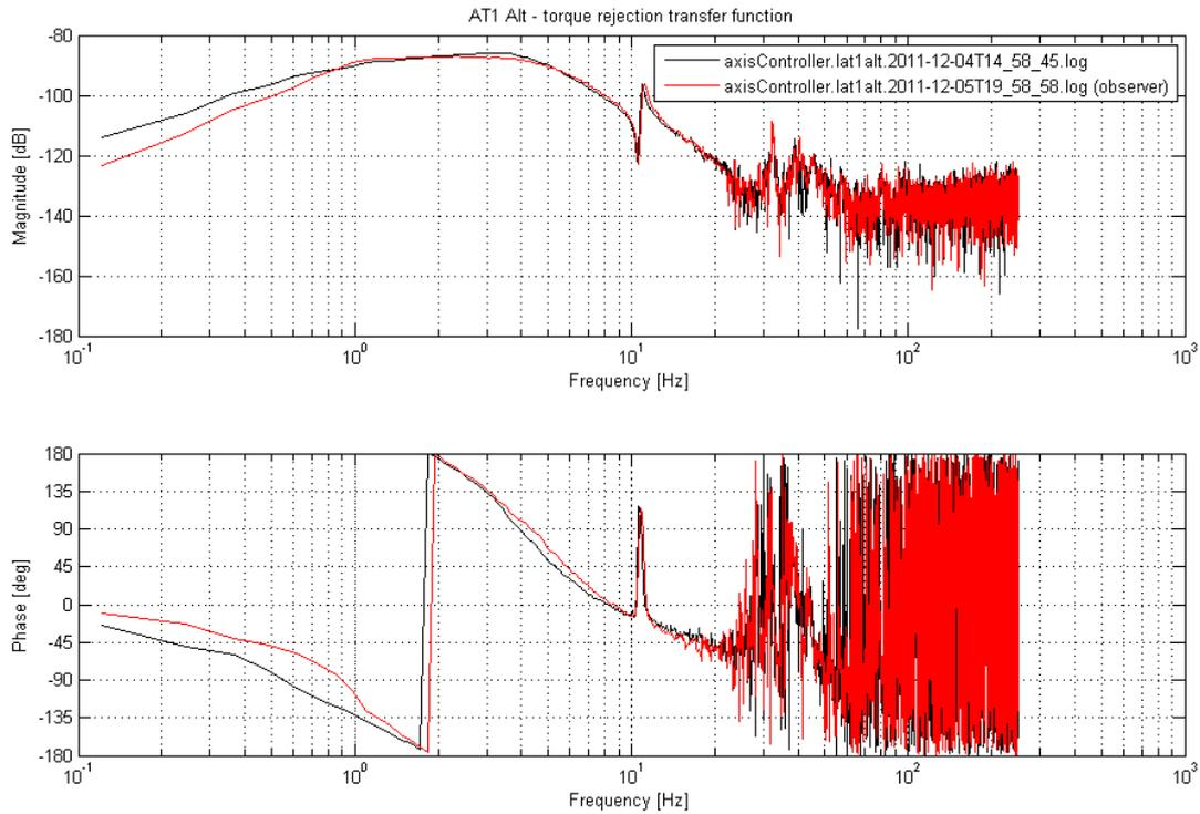
Figure 8. AT1 Altitude torque rejection transfer function improvement with observer.
