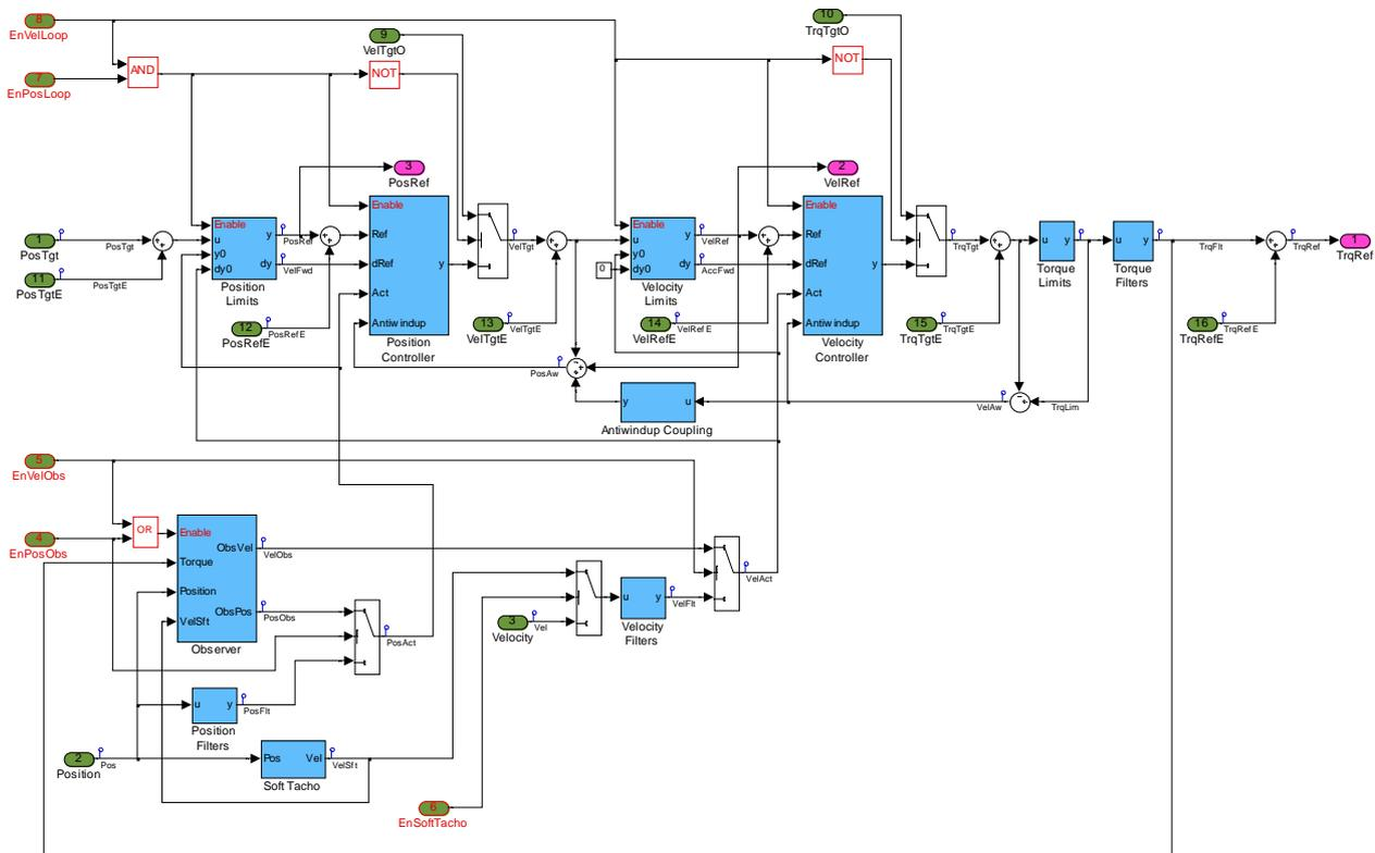
Figure 1. Simulink model of the axis controller.
