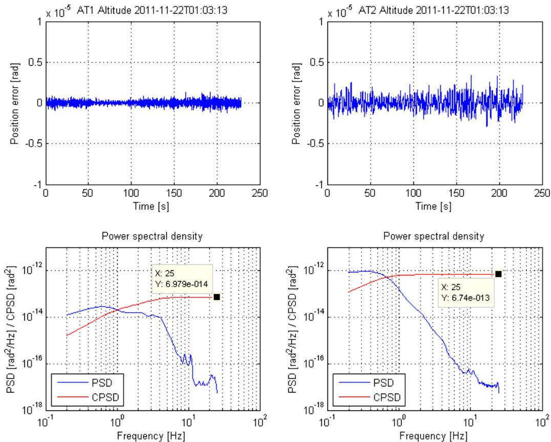
Figure 4. Comparison of performance in wind: AT1 with new software (left), AT2 with old software (right).
