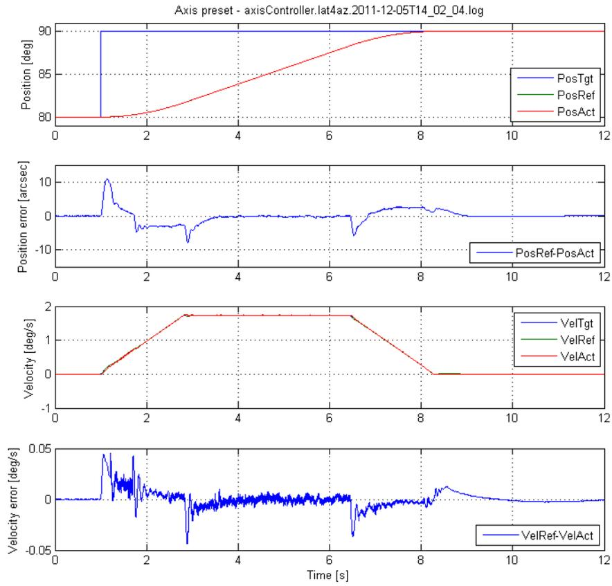
Figure 5. Behaviour during preset (slewing).
