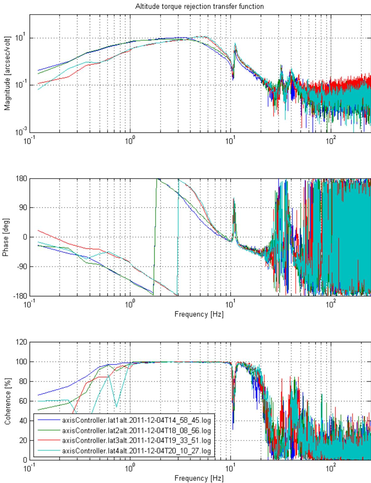
Figure 7. Measurement of torque rejection transfer function for the four VLT Auxiliary Telescopes.
