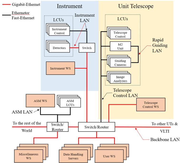
Figure 1: Network, workstations, LCUs: logical lay-out of the VLT LANs
