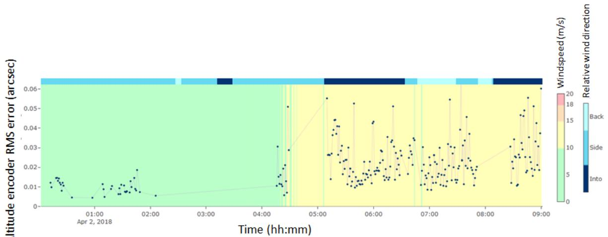
Figure 11: UT1 altitude axis encoder error versus wind speed and direction
