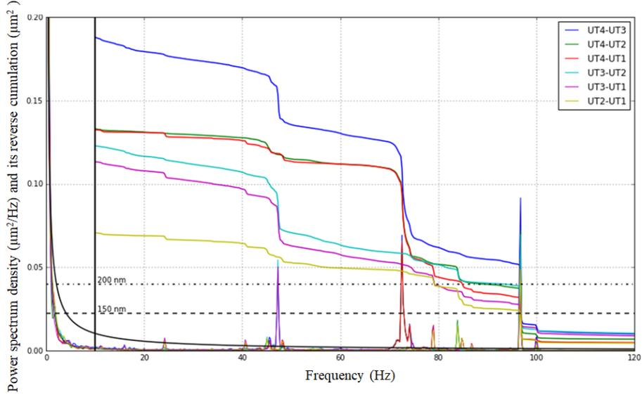
Figure 16: VLT baseline optical path difference: cumulative power density spectra during May 2016
