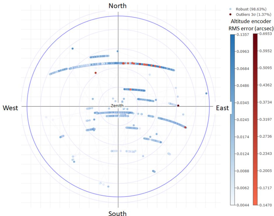
Figure 9: UT1 altitude axis encoder error
