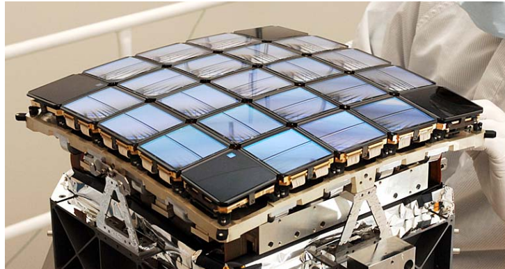
Figure 4: Image of Kepler focal plane, employing a CCD detector mosaic on a curved spherical substrate [3] Reproduced with permission from authors
