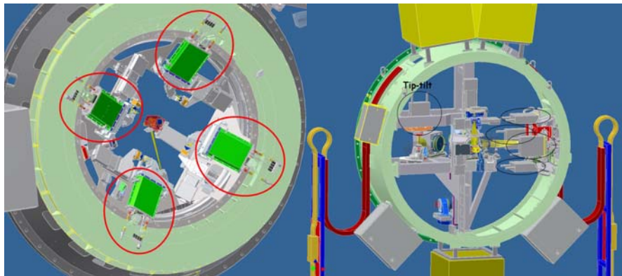
Figure 6: On the left GRAAL with 4 AOWFS heads and on the right GALACSI with one additional tip-tilt camera.
