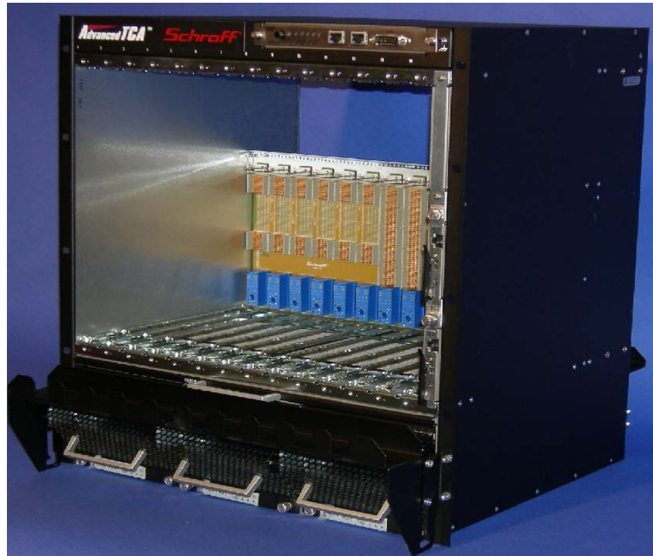
ATCA shelf with cooling fans
