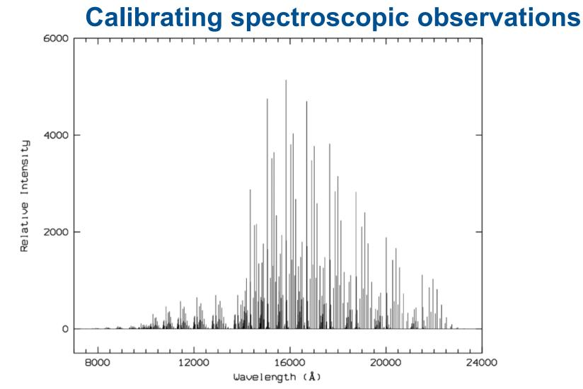
Usual procedure in visible and infrared: arc lamps (emission-line calibration source in the instrument)
