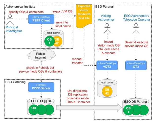
OBs are essential components of the ESO Dataflow System, involving different tools, processes, databases and sites
