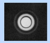
→ Two telescopes of 4 and 8m will resolve an angle separation of 3.1 10<sup>-2</sup> and 1.6 10<sup>-2</sup> arcsec
