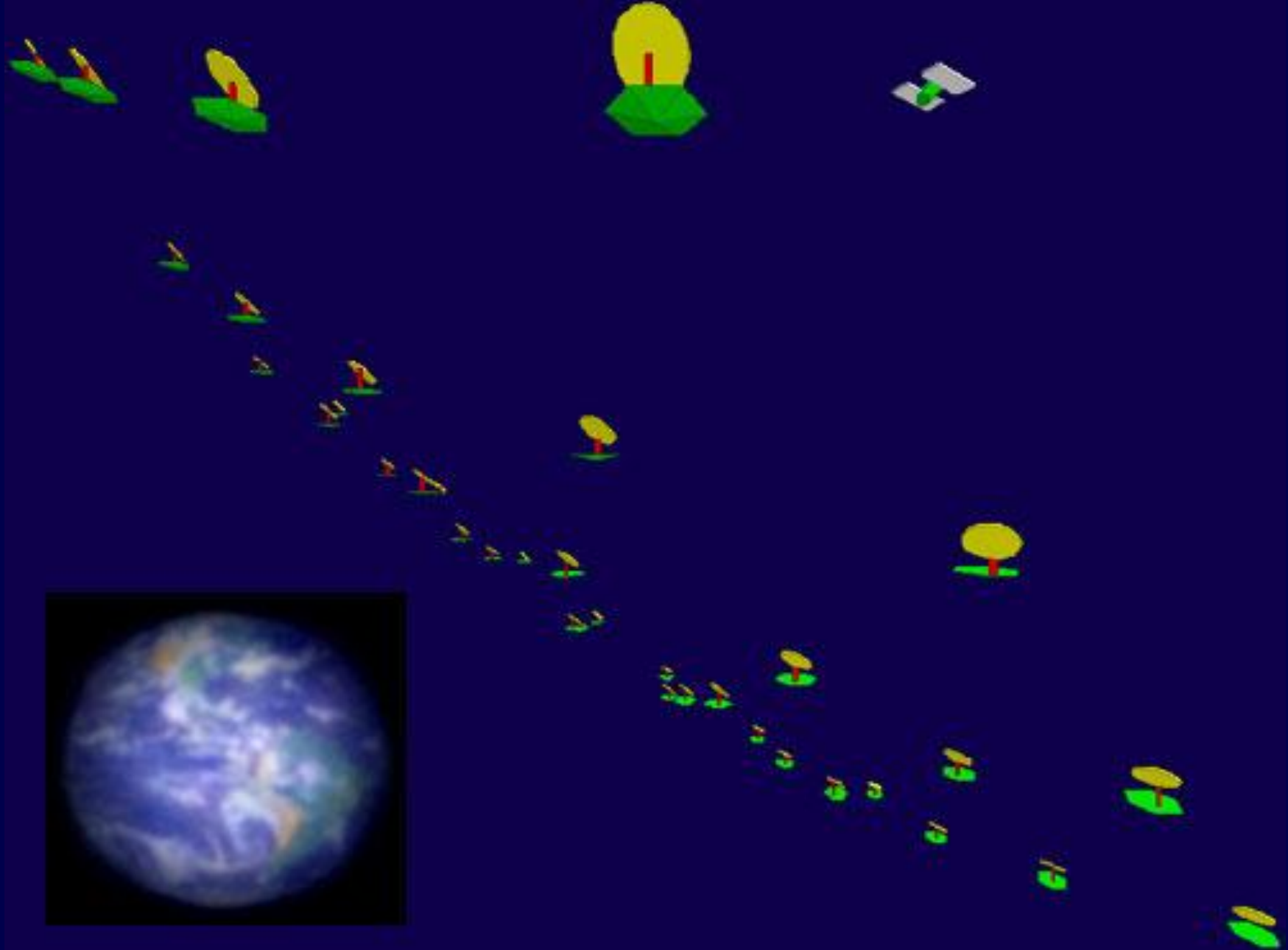
Exo-Earth Imager (150 km baseline space interferometer) with a simulated 30-min exposure of Earth at 3 parsec distance. (Antoine Labeyrie)
