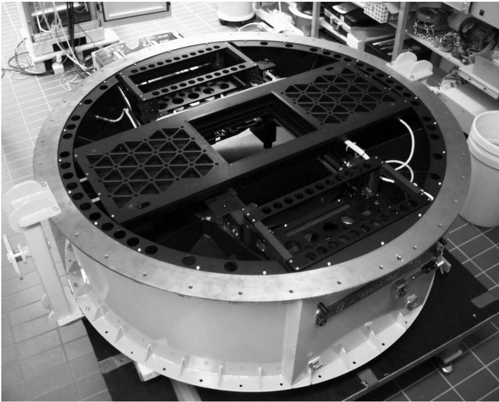
**Figure 3.** *The 1.5m diameter housing structure with integrated storage magazines for filters (in the upper and lower part of the photo) and shutter (structure going from left to right). Each magazine can be filled with up to 6 filters.*
