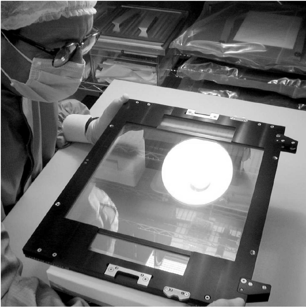
**Figure 6.** The  $r'$  filter in optical lab of the manufacturer SAGEM. The overall size of the frame is  $424 \times 326$ mm. The total mass is 6kg. In the center the  $268 \times 268$  main field of view (science filter). Below and above science the auxiliary filters for guiding and image analysis are located.
