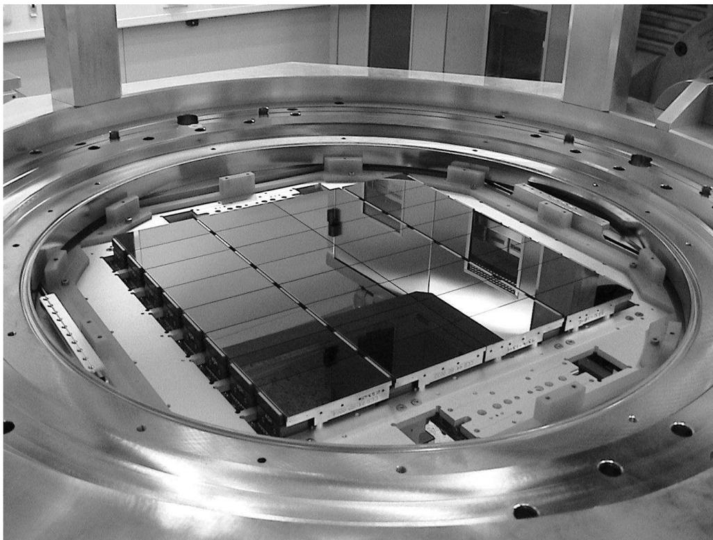
**Figure 1.** *The OmegaCAM focal plane in the laboratory, populated with dummy CCDs. This arrangement minimizes the amount of dead space between devices, given the constraints imposed by connecting the read-out ports. In the VST the array covers a 1x1 degree area. In addition to the 32 CCDs shown here, in the periphery the mounting holes can be seen for the four auxiliary detectors—two of these are for autoguiding, and the other two for image analysis.*
