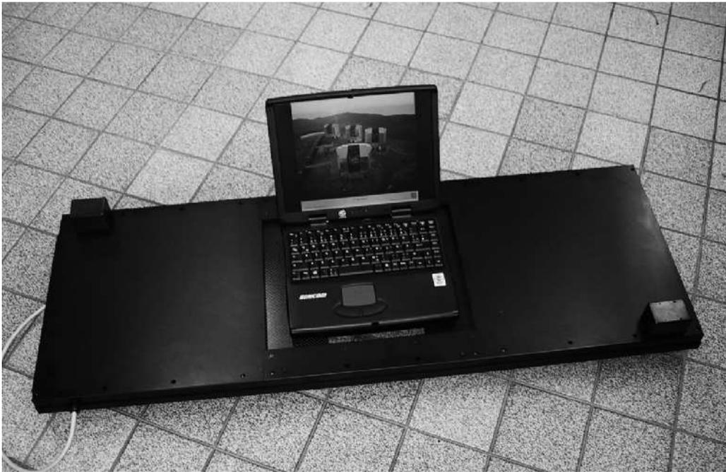
**Figure 4.** *The OmegaCAM exposure shutter. The aperture size is  $370 \times 292$ mm, the shortest possible exposure time is smaller than 1msec, the deviations of the effective exposure time from pixel to pixel (homogeneity) are smaller than  $\pm 0.3\%$  for a 0.2sec exposure, the exposure time accuracy is about 0.3msec. The laptop is shown for scale.*
