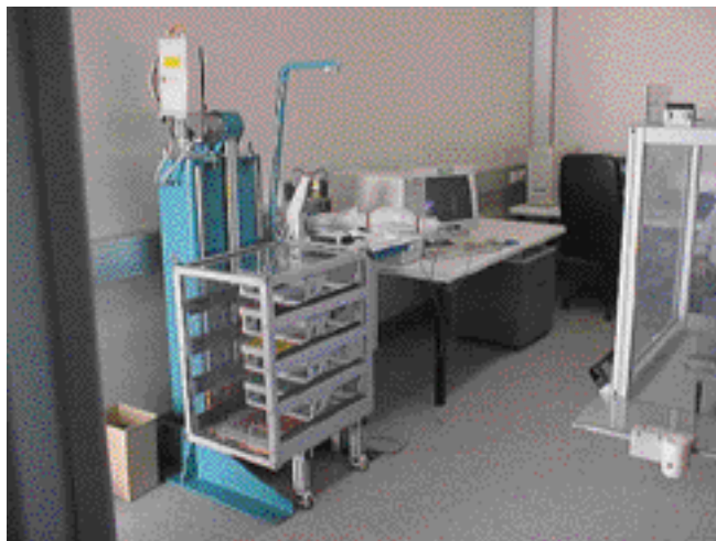
Figure 6: The Instrument Cabinet Robot. The four Instrument Cabinets corresponding to the four channels of VIMOS (or NIRMOS) are inserted in the stand.
