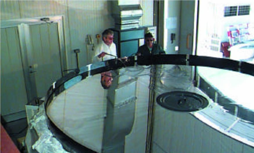
Figure 2: The NTT main mirror being rinsed with distilled water. The last washing step before drying the mirror surface.
