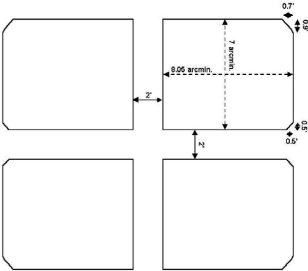
Figure 1: VIMOS field as projected on the sky, each quadrant has a field  $7 \times 8 \text{ arcmin}^2$ , for a total field of  $224 \text{ arcmin}^2$ .
