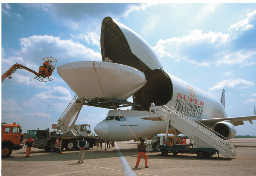
On 16 May 2003, at the airport of Milano Malpensa, the receiver cabin and reflector backup structure (BUS) of the Alcatel/EIE Antenna prototype were loaded on the special Airbus A 300 transporter ("Beluga") for shipment to Albuquerque airport (NM, USA) en route to their final destination, the VLA site in Socorro. Both cabin and BUS were manufactured in Italy and are made of carbon fibre reinforced plastic (CFRP) based on a design by the European Industrial Engineering (I) under the supervision of Alcatel Space Industries (F).
