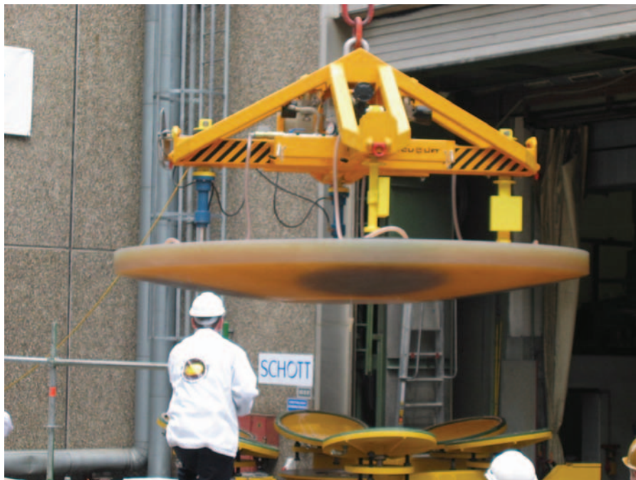
Figure 8: Preparing the f/1 meniscus primary to leave Schott.
