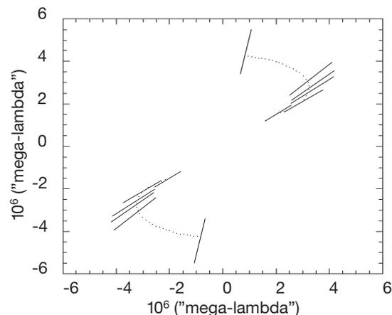
**Figure 3:** The  $uv$ -coverage of the observations in P73 is shown. The dotted line indicates the change of projected baseline length due to earth rotation. Whereas the earth rotation curve is calculated at a central wavelength of  $10.34\ \mu\text{m}$  the solid lines are showing the  $uv$ -coverage of each dispersed, calibrated visibility dataset.
