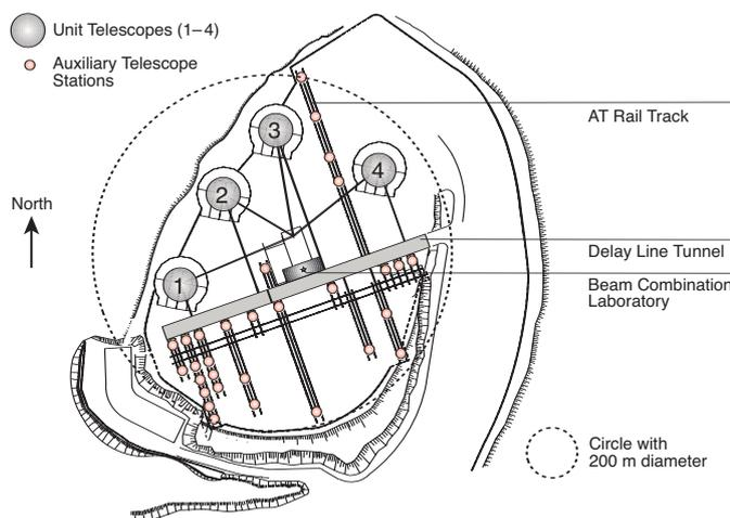
**Figure 1:** View of the Paranal platform with the position of the four fixed 8 m VLT Unit Telescopes (UTs) and the 30 positions for the movable 1.8 m Auxiliary Telescopes (ATs). Compare with the aerial view in Figure 2 and the recent photograph in Figure 3.
