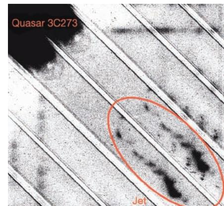
Figure 10 (below): Polarization data of the quasar 3C273 jet. NACO has been rotated to align the jet with the Wollaston stripe mask. The retarder plate can be used to turn the polarization direction in order to derive the polarization map (image prepared by Sebastian Jester).
