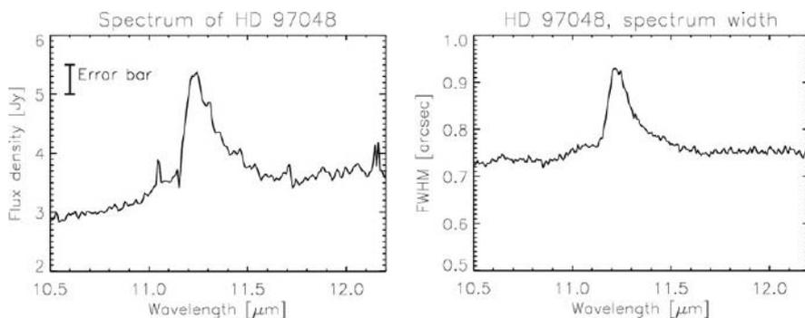
Figure 5: Left: Observed spectrum of HD 97048 around 11.4  $\mu\text{m}$  in the long-slit low-resolution mode of VISIR. Right: The measured spatial full width at half maximum of the HD 97048 spectrum as a function of wavelength. The PAH emission at 11.3  $\mu\text{m}$  is spatially more extended than the continuum and confirms the spatial extension of the image seen in Figure 4.
