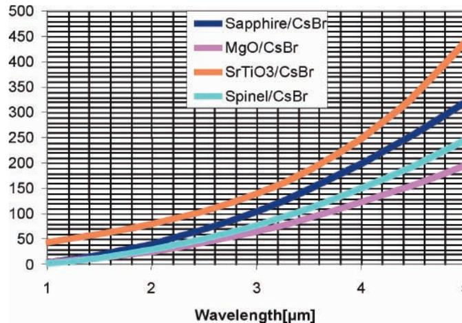
Figure 8: Spectral resolving power over the CONICA NIR range provided by prisms of different composition.
