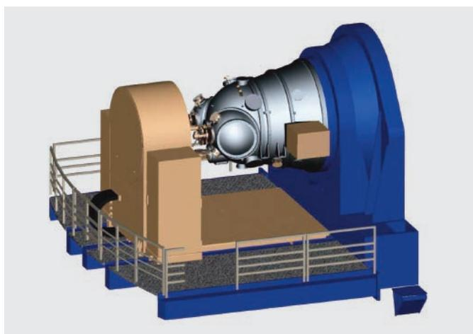
pact focal plane with a cross-shaped gap of 2.7 mm or 15 arcsec. The detectors will be assembled in a package developed by GLScientific which allows all 32 channels per detector to be read out. A CAD drawing of the assembly is shown in Figure 3.
