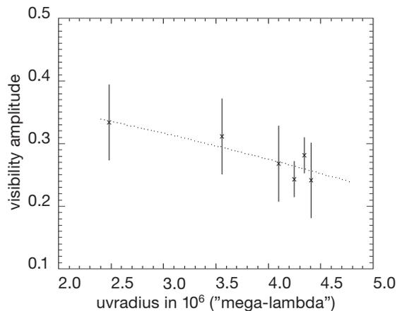
**Figure 2:** Median 8–12  $\mu\text{m}$  visibility of IRS 3 as a function of projected baseline length. Currently the uncertainty of the visibilities is above all affected by the instrument calibration. Therefore the errors are given by the standard deviation of the instrument calibration over the entire night.
