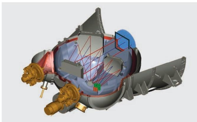
Figure 5: This drawing shows HAWK-I attached to the Nasmyth adapter (blue). The cable de-rotator (brown) is also shown.
