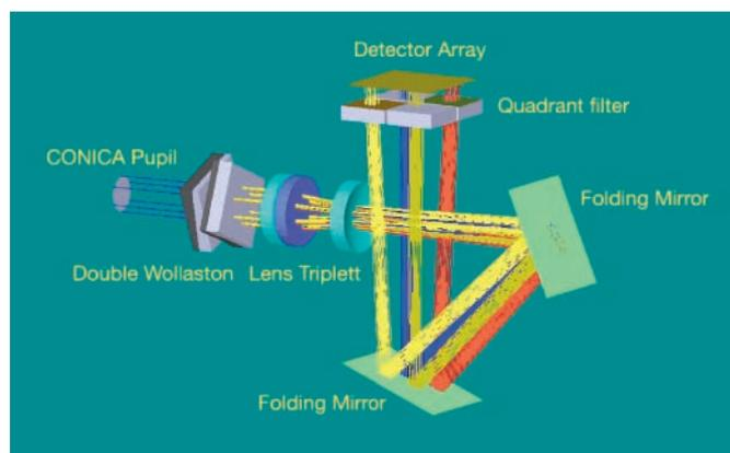
Figure 2: SDI optical concept. A double Wollaston prism splits the beam into four which are imaged through different filters located on the either side of the *H*-band methane feature at 1.62  $\mu\text{m}$ .
