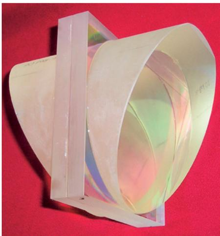
Figure 2: The VPH grism as hosted inside the new mounting.
