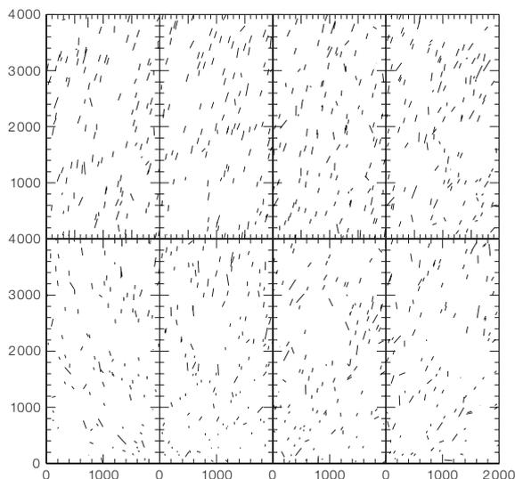
**Figure 2:** A typical ellipticity distribution of stellar objects for a WFI exposure with a seeing of 1''. WFI is a CCD mosaic camera with 4 × 2 chips each having 2K × 4K image pixels. The total field of view of the camera is 34' × 33'. The sticks indicate the orientation and length of the stellar ellipticity in the field. No stellar image has an ellipticity larger than 2.5% (corresponding to an ellipse with an axis ratio of ~ 0.95) and the PSF is smooth over the whole field of view.
