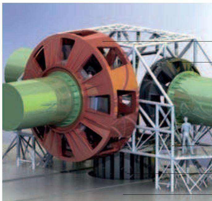
Figure 7 (below). CAD rendering of a Nasmyth platform populated with indicative instrument volumes and the prefocal unit.
