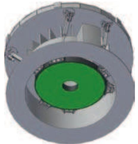
Figure 5 (above and right). Two preliminary designs for the M4 deformable mirror unit.
