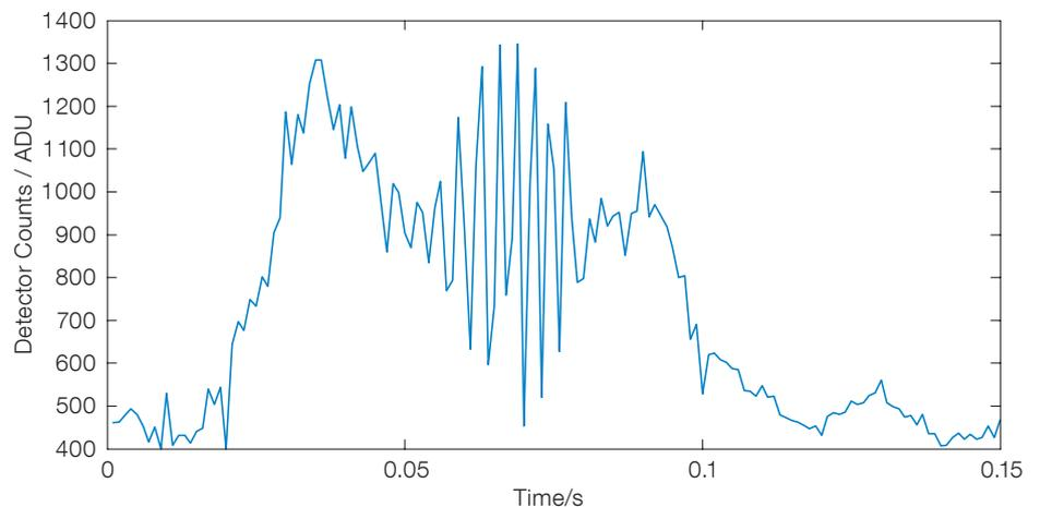
Figure 2. First fringes for PRIMA, obtained on Fringe Sensor Unit A on 3 September 2008, observing the star HD 19349 with two ATs separated by 32 m at VLTI stations G0 and G2.
