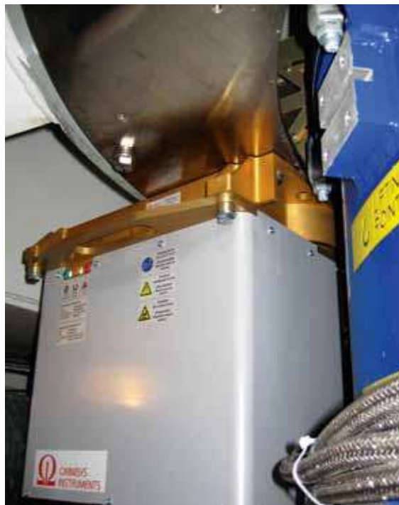
Figure 11. First production water vapour radiometer mounted inside an ALMA antenna.
