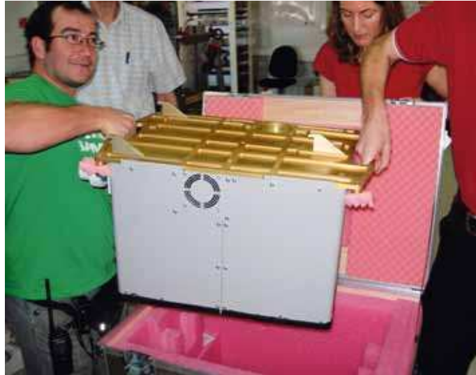
Figure 10. First production water vapour radiometer being unpacked after arrival at the ALMA Operations Support Facility.
