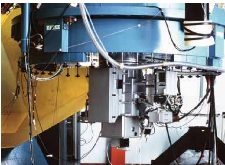
Figure 5. The F/35 IRAC1 camera mounted at the MPG/ESO 2.2-metre telescope.
