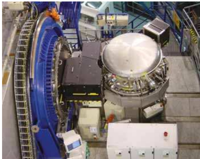
Figure 7. CRIRES, last of the first generation instruments on the VLT (UT1). The black box to the left houses the adaptive optics system and the vacuum vessel contains the 1–5 \mu\text{m} , R = 100\,000 , cryogenically cooled echelle spectrograph.
