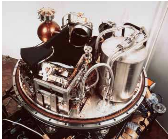
Figure 4. IRSPEC used for medium resolution 1–5 \mu\text{m} spectroscopy at the 3.6-metre and NTT telescopes. Its novel design includes the use of a warm bench to support all the optical units that are cryogenically cooled by a continuous flow of liquid nitrogen from the internal tank on the right. It was also the first infrared spectrograph equipped with a monolithic infrared array detector — initially a 1 x 32 linear array of InSb diodes (cooled by liquid/solid nitrogen in the small copper dewar) and later a 2D 58 x 62 InSb array (cooled by the first mechanical closed cycle cooler used at ESO). In operation, the instrument was enclosed by a dome-shaped cover and evacuated.
