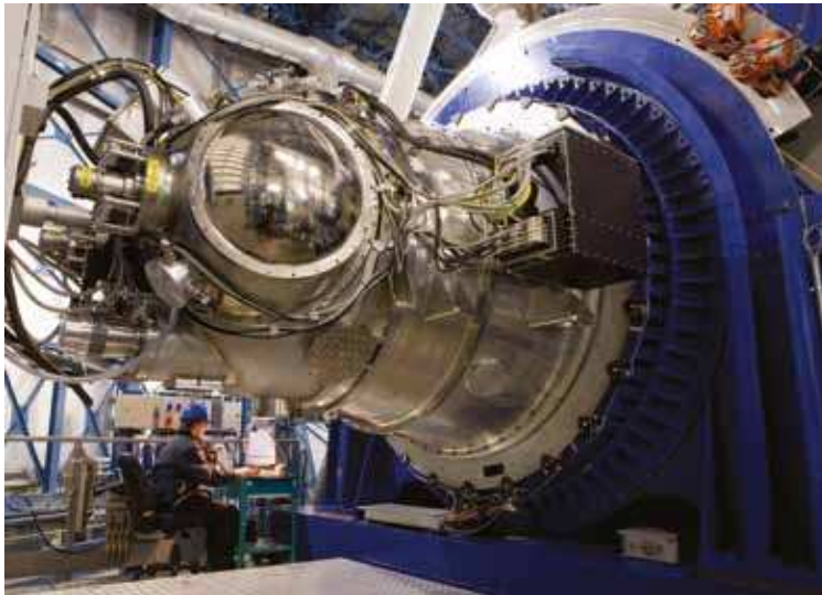
Figure 8. HAWK-I on the VLT (UT4). This near-infrared camera is equipped with four 2k x 2k Hawaii 2 Rockwell/Teledyne arrays. Although employing mirror optics to image its large 7.5 x 7.5 arcminute field of view with maximum optical efficiency it appears overly large here due to the artistic choices of lens and viewing angle.
