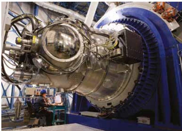
**Figure 8.** HAWK-I on the VLT (UT4). This near-infrared camera is equipped with four 2k x 2k Hawaii 2 Rockwell/Teledyne arrays. Although employing mirror optics to image its large 7.5 x 7.5 arcminute field of view with maximum optical efficiency it appears overly large here due to the artistic choices of lens and viewing angle.
