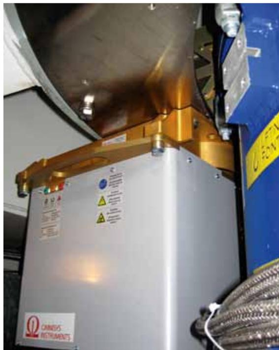
Figure 11. First production water vapour radiometer mounted inside an ALMA antenna.
