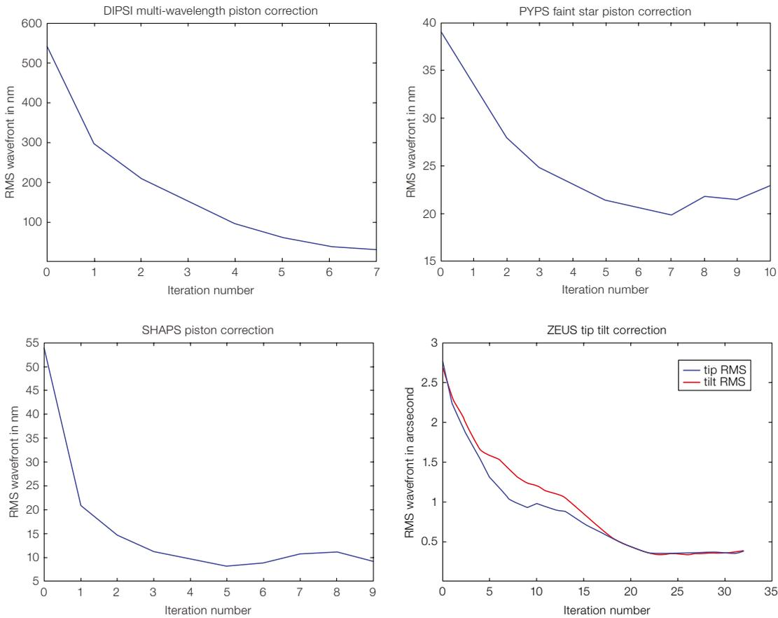
Figure 7. The resulting rms error on closed-loop corrections for the four OPSs: (a) DIPSI, piston correction using multi- $\lambda$  technique; (b) PYPS, piston correction with a faint star (magnitude 18); (c) SHAPS, piston correction with a bright star; (d) ZEUS, tip and tilt correction.
