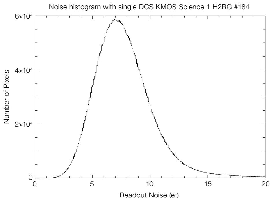
**Figure 4.** Noise histogram for single double-correlated readout of a 2K x 2K HgCdTe substrate-removed  $\lambda_c = 2.5 \mu\text{m}$  Hawaii-2RG array (KMOS science-grade array #1). The noise distribution peaks at 6.9 electrons (rms).
