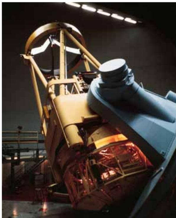
Figure 2. (Right) F/35 chopping secondary mirror on the 3.6-metre telescope.
