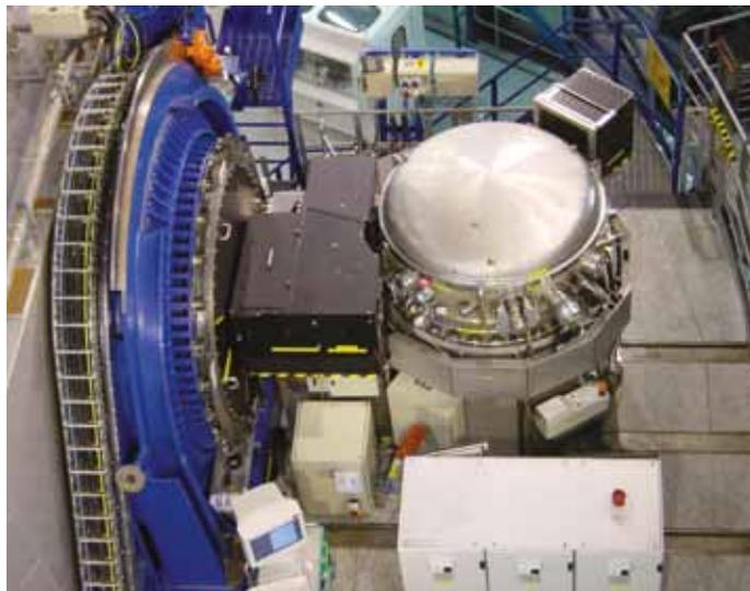
Figure 7. CRILES, last of the first generation instruments on the VLT (UT1). The black box to the left houses the adaptive optics system and the vacuum vessel contains the 1–5  $\mu\text{m}$ ,  $R = 100\,000$ , cryogenically cooled echelle spectrograph.
