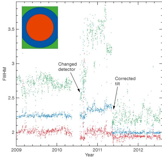
**Figure 2.** Evolution of the image FWHM in pixels since 1 January 2009 for VIMOS channel 4. The red points correspond to the average FWHM of the pinholes within 800 pixels of the centre; blue between 800 and 1200 pixels and green to those beyond 1200 pixels (see the schematic of the regions used on the detector to the upper left). Arrows mark when the detector was changed and the tilt corrected.
