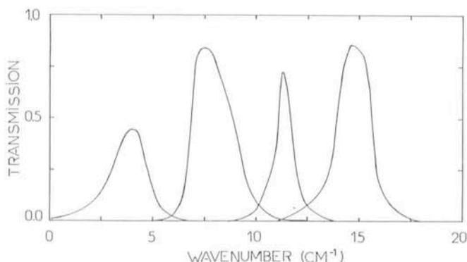
Fig. 2: Spectral shape of the band-pass filters used for astronomical sources.
