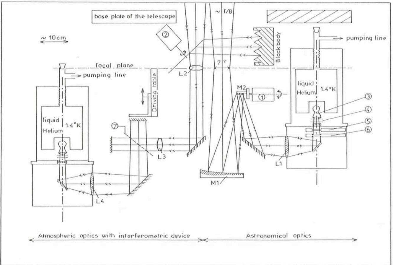
Fig. 1: Optical schema of the millimeter photometer with sky emission spectral measurement. ① Scanner motor for sky modulation; ② Chopper; ③ Detector with light-cone; ④ Cold filters; ⑤ & ⑥ Filter wheels; ⑦ Beam splitter; M1 Parabolic mirror; M2 Wobbling mirror for sky modulation; L1 & L4 Quartz lenses; L2 & L3 TPX lenses.
