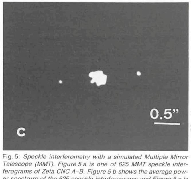
Fig. 5: Speckle interferometry with a simulated Multiple Mirror Telescope (MMT). Figure 5 a is one of 625 MMT speckle interferograms of Zeta CNC A-B. Figure 5 b shows the average power spectrum of the 625 speckle interferograms and Figure 5 c is the reconstructed autocorrelation of Zeta CNC A-B (separation =  $0^{\circ}.81$ ).
