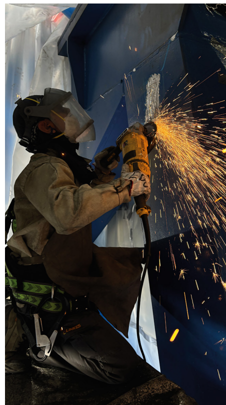
Figure 6. Grinding the surface of the telescope structure to ensure a smooth interface.
