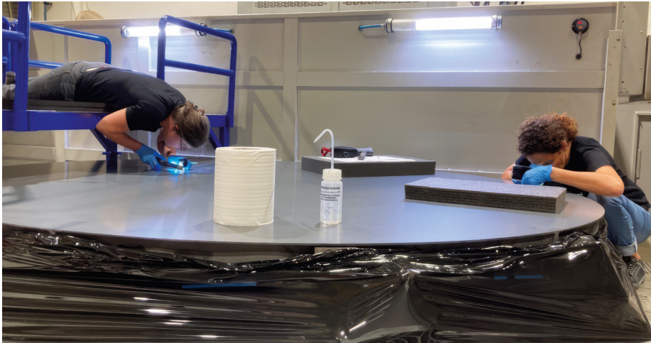
Figure 9. The M5 Blank under inspection after grinding of the front face by Mersen Boostec.
