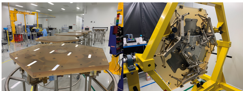
Figure 1. M1 segment polishing at Safran. Left: the segments are waiting for final inspection.
