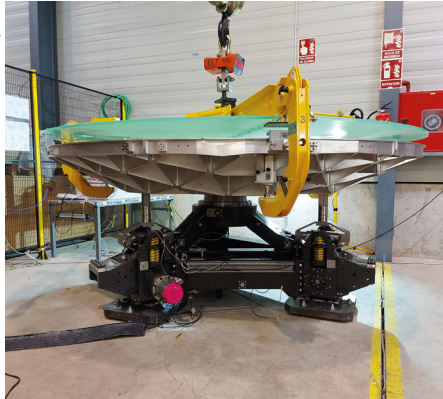
Figure 8. The M5 Cell with the dummy mirror.
