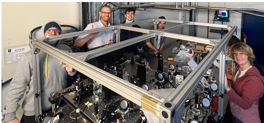
Figure 2. Core Asgard team members installing the outer enclosure in the VLTI laboratory on the visitor table — once panels were in place, it became more difficult to see inside in a single photo!
