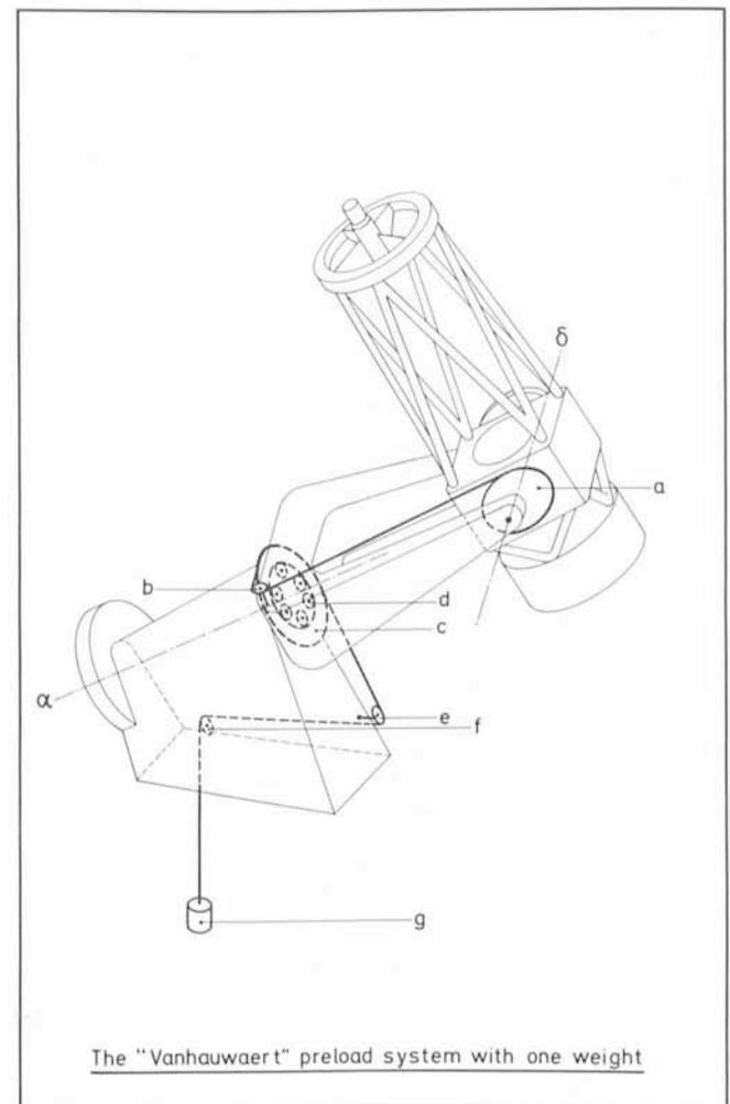
The "Vanhauwaert" preload system with one weight
