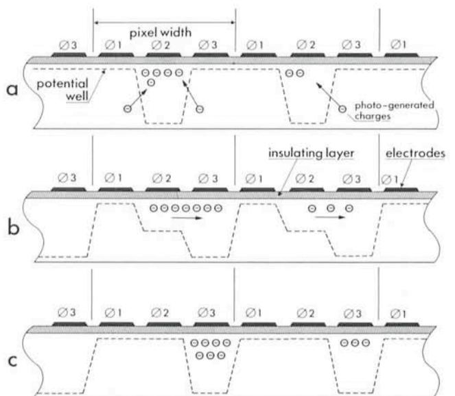
Fig. 1: Potential well structure generated by the overlaying electrodes along a column of a 3-phase CCD. (a) Static potential wells during integration; (b) and (c) charge transfer process during image read-out.
