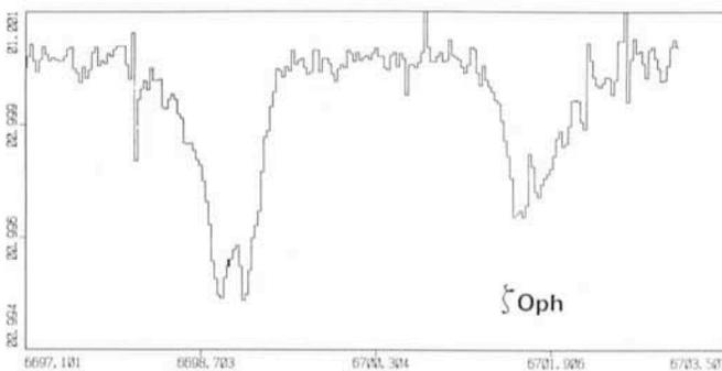
Fig. 5: Possible new interstellar absorption lines due to the molecule  $\text{CS}^+$  toward  $\zeta$  Oph. Same spectrum as in Fig. 4. The equivalent widths of the two features are of the order of 3 and 2 mÅ.
