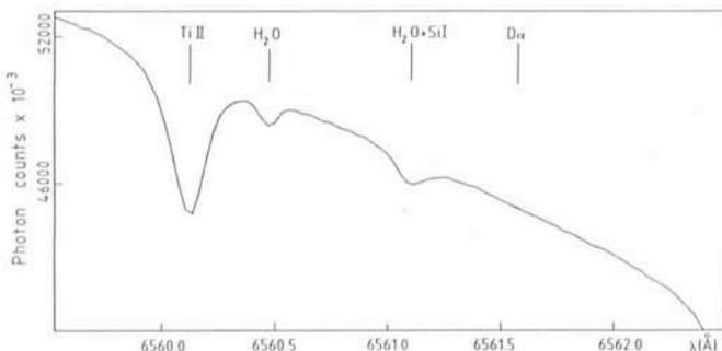
Fig. 2: Enlarged portion of the  $H\alpha$  blue wing in the CES spectrum of Canopus, with some relevant stellar and atmospheric water lines marked. 29 exposures have been added and the actual signal-to-noise ratio is around 3700.
