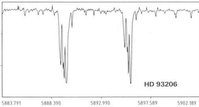
Fig. 1: The interstellar Na I D lines toward HD 93206 in the Carina region, taken with the CES + Reticon at  $10^5$  resolving power in one hour. The wavelength calibration is based as usual on neon and thorium lines and/or on a standard star. Clearly 5 components are detected; all very weak lines spread over the spectrum are due to atmospheric water absorptions.
