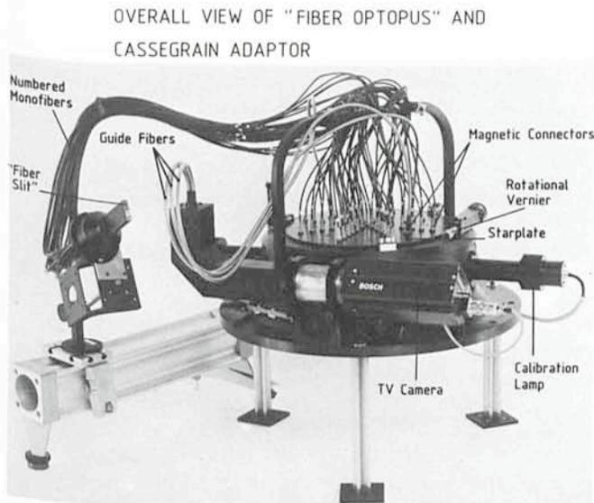
Fig. 2: Photographic view of the Optopus and associated hardware, before installation on La Silla. The metallic housing attached to the TV camera contains transfer optics for the guidestar images.
