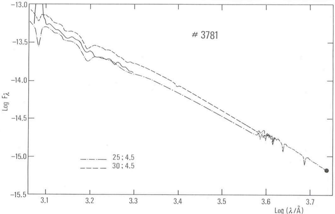
Fig. 2: By fitting IUE spectra to the observed  $V$  magnitude, reliable evaluations of effective temperatures are obtained. The dot indicates the flux corresponding to the visual magnitude; the IUE SWP spectrum (after rebinning in bands of 40 Å) is also shown (continuous line). The two comparison spectra are taken from Kurucz model atmospheres at the indicated temperatures (in units of 1000°K) and gravities (logarithm of).
