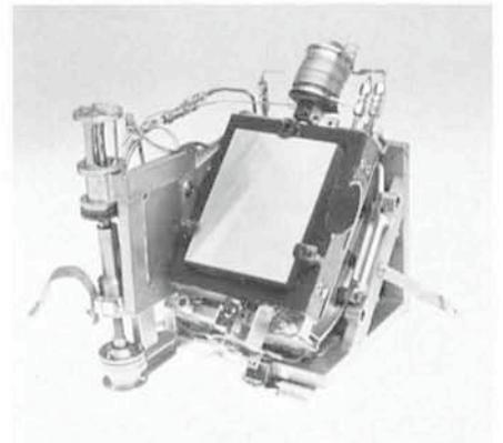
Figure 3: The grating cradle support which permits interchange of the two back to back gratings and precision scanning about their ruled surfaces.
