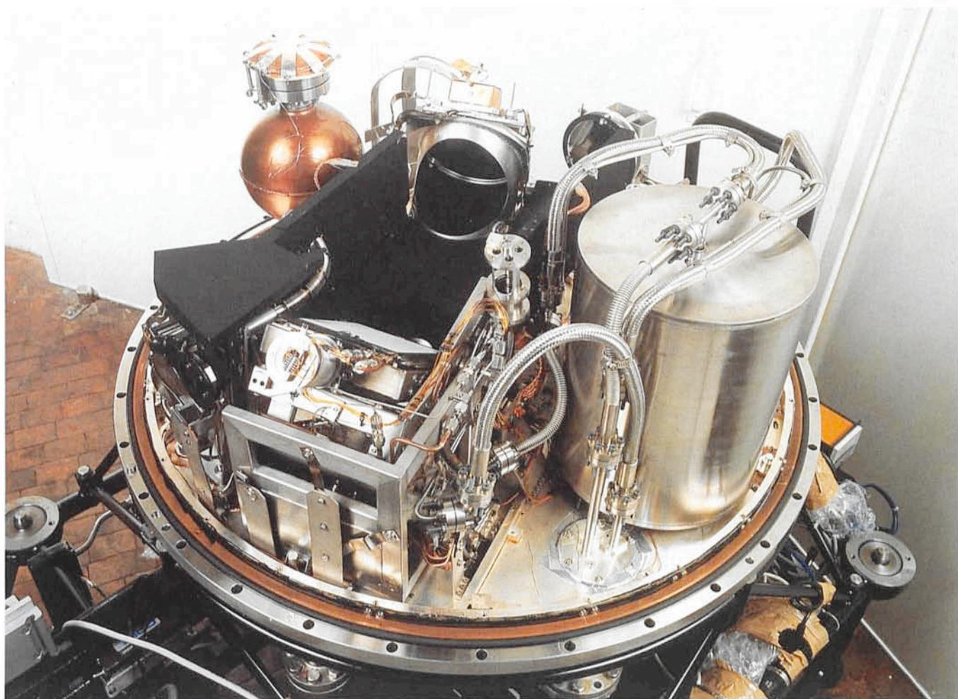
Figure 1: IRSPEC with the upper parts of its radiation shield and vacuum vessel removed. The spectrometer is cooled by a continuous flow of liquid  $\text{N}_2$  supplied either by the internal reservoir on the right or from an external tank while the detector array is cooled by solid  $\text{N}_2$  contained in the copper cryostat (upper left).
