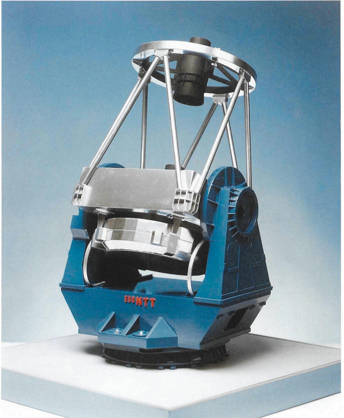
*Model of the ESO New Technology Telescope.*
