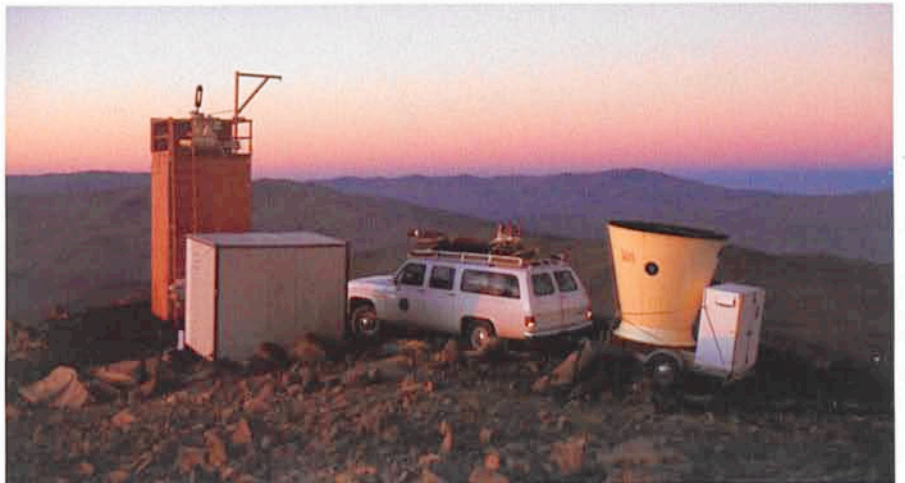
Figure 1: Trailed Sodar, Seeing monitor and control room shelter.
