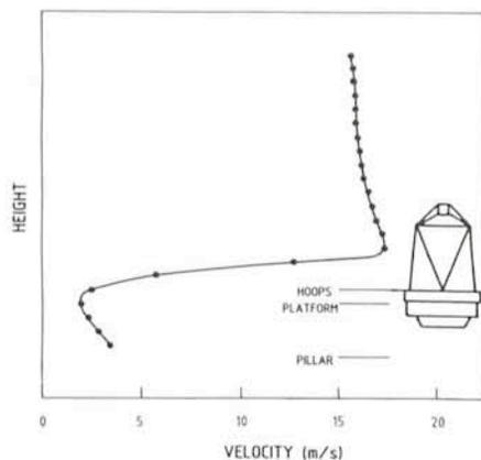
Figure 5: Wind velocity profile along the azimuth axis measured during wind tunnel tests.
