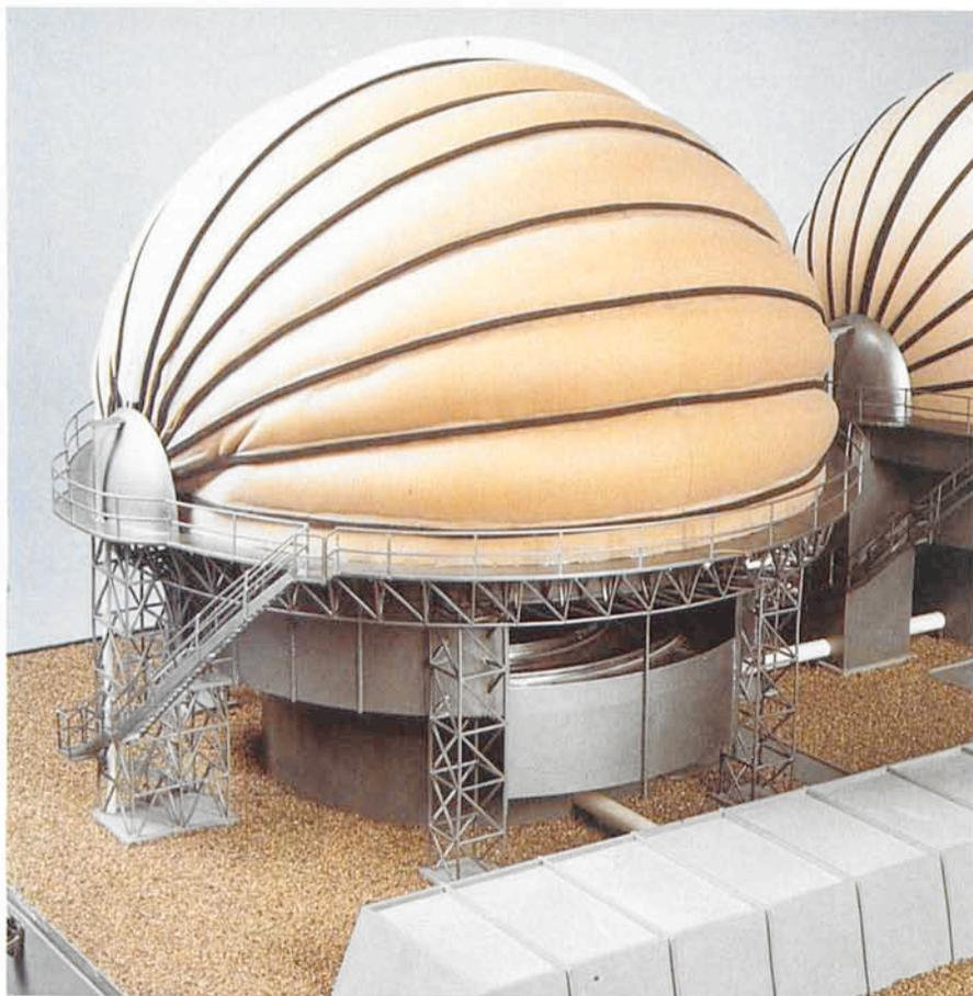
Figure 3: The latest enclosure design for the VLT unit telescopes. The sliding door in the recess is used for natural ventilation. From another one at the opposite end it is possible to take the primary mirror out for aluminization.
