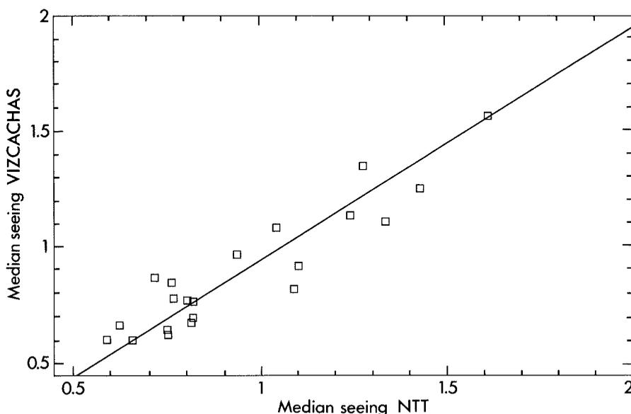
Figure 2: *Night to night comparison between the seeing recorded at the NTT and Vizcachas.*
