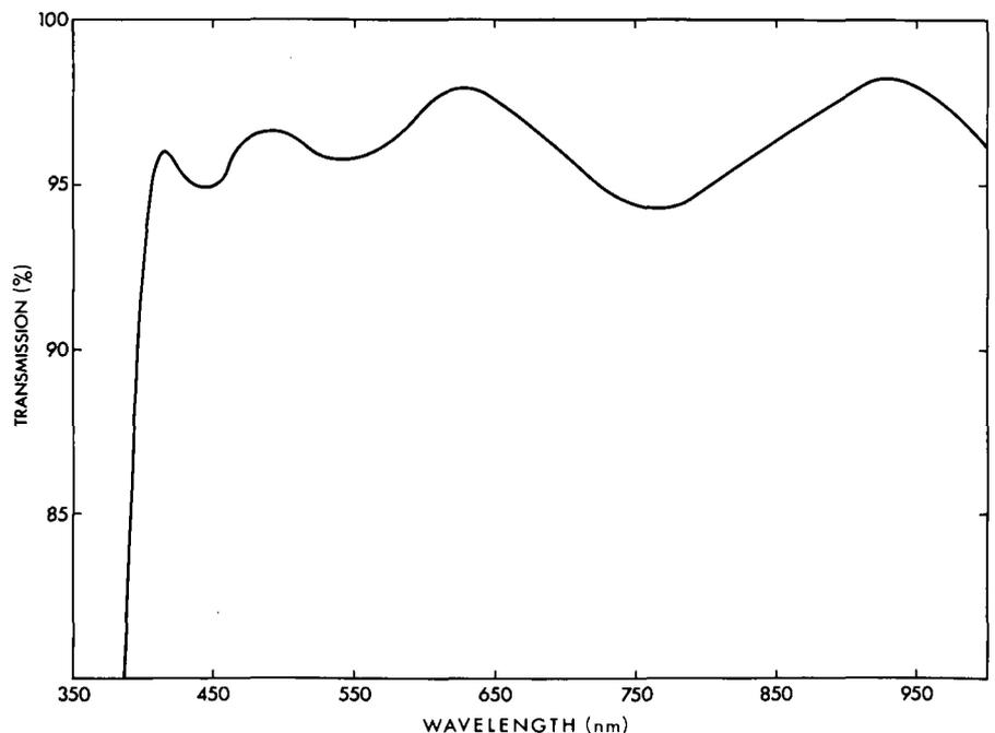
Figure 1: The transmission of the red collimator (consisting of two cemented doublets) in single pass. It is used in double pass, so the total efficiency in the range 4000–10000  $\text{\AA}$  will be over 90%, still better than a single aluminium mirror.
